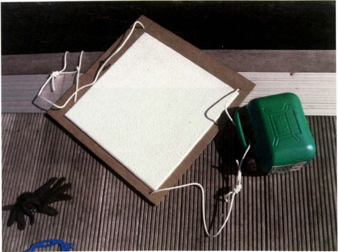
Figure 5.2. Experimental set-up. The green plastic container is filled with sand to act as a weight.
