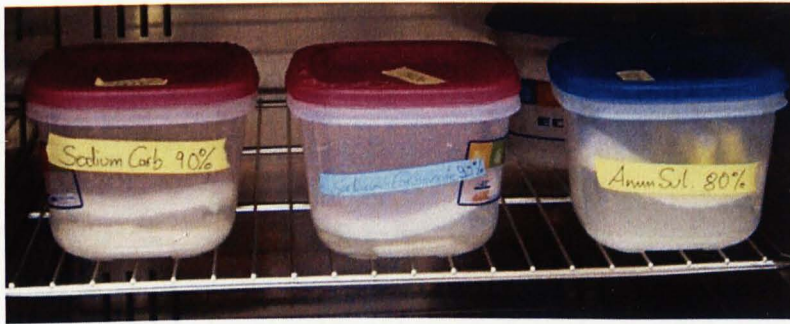
Figure 5.3a: Airtight plastic boxes (humidity chambers) containing saturated salt solutions creating different humidities
