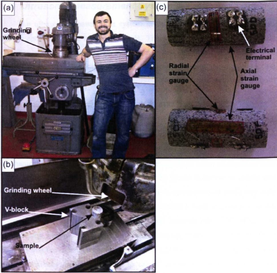
Figure 2-12. Squaring and surface finishing of cores. a) Grinding machine. b) Cored sample fixed in V-block. c) Radial and axial strain gauge glued to core.
