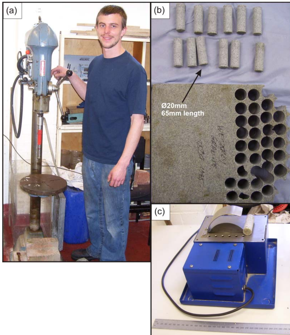
Figure 2-11. Coring and cutting the ends of a rock sample. a) Coring drill. b) Cores from a Westerly granite sample. c) Diamond blade saw
