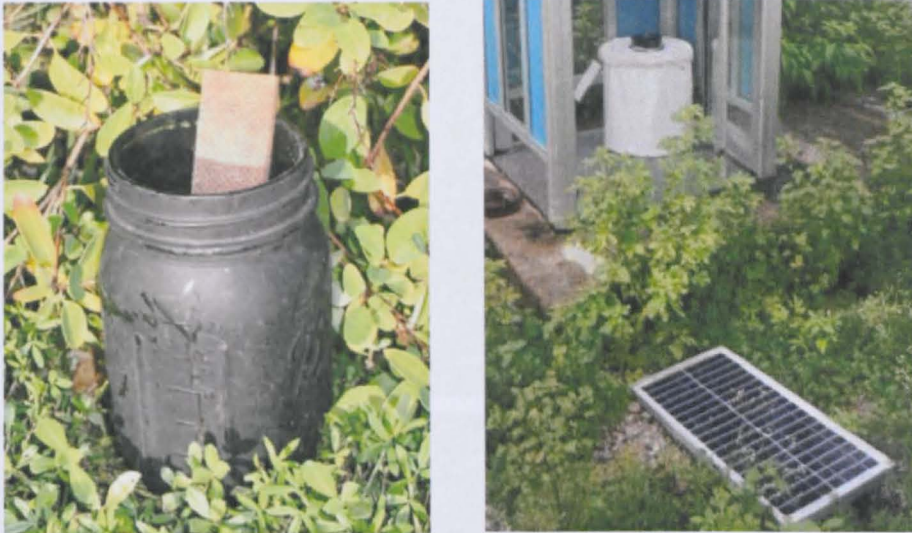
Figure 5.3 Ovitrap and BG sentinel traps used for monitoring during the RIDL field trials. The BG sentinel trap is powered by a battery charged by a solar panel.
