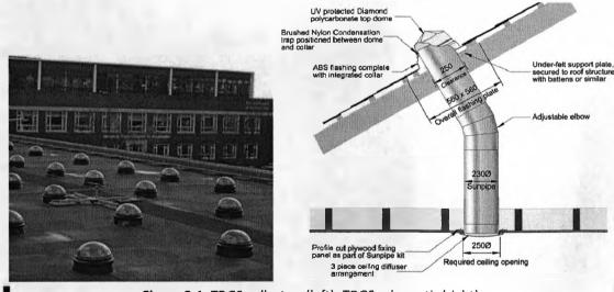
Figure 3.1: TDGS collectors (left); TDGS schematic (right).
