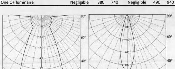
Figure 7.8: Parans luminaire polar curves, (Left): L1-large (Nadir luminous intensity 273cd/1000 lumens), (Right): L1-small (Nadir luminous intensity 1220Cd/1000 lumens)
