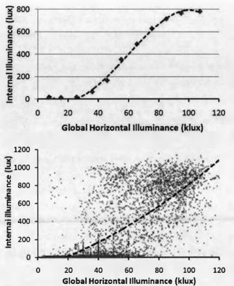
Figure 7.4: Relationship of external global horizontal illuminance to average value of nadir illuminance delivered by Parans system
