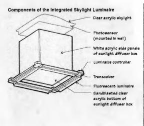
*Figure 3.7: Components of the ISL* (above); *An installation of ISL in a warehouse* (right).
