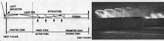
Figure 3.3: Light pipe section (left); Model of the interior LCP light diffuser (right).
