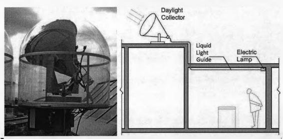
Figure 3.5: Solux system collectors (left); Solux system schematic (right).
