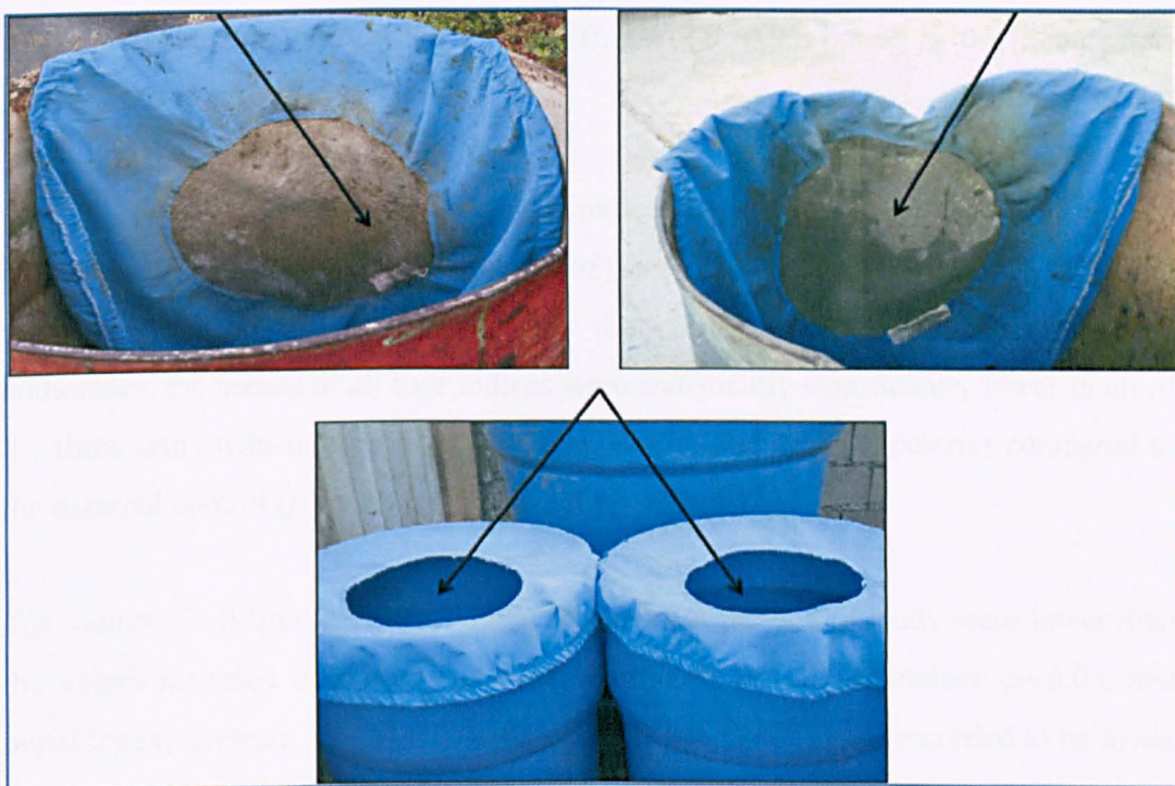
Figure 3.10. Physical deterioration in covers in the study site, after fourteen months of use (photographs from January 2008).
