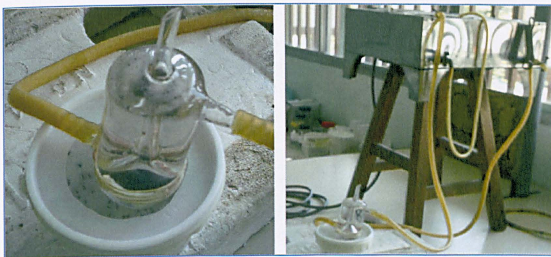
Figure 5.3. Artificial membrane feeding system for Aedes aegypti, with fresh human blood and newborn chick skin membranes.
