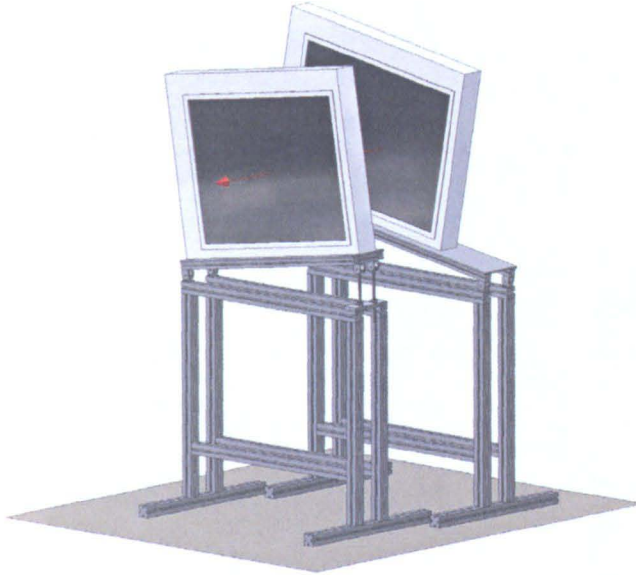
Figure 3.11: The Proton Drift Chamber detectors with their supporting structures and a depiction of a perpendicular proton track. The distance from the base of the structure to the centre of the active area (indicated by the proton track in red) is approximately 2m.
