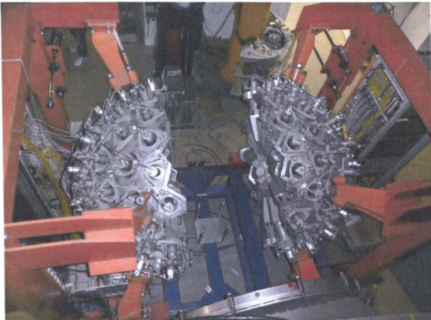
Figure 3.8: The Crystal Ball detector opened to allow the positioning of the target chamber.
