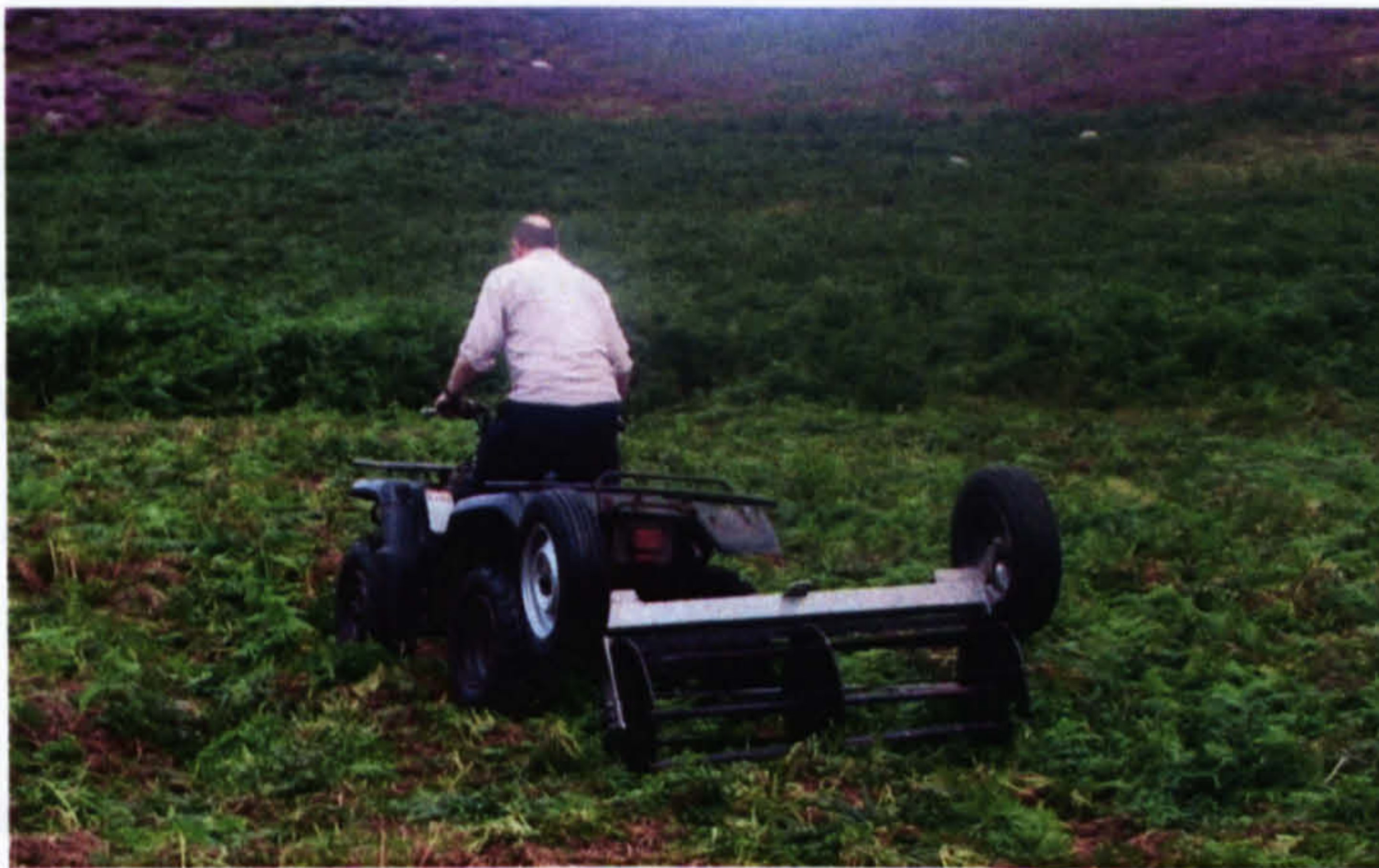
Fig. 1. Bracken being bruised by a bruiser trailed on an ATV.
