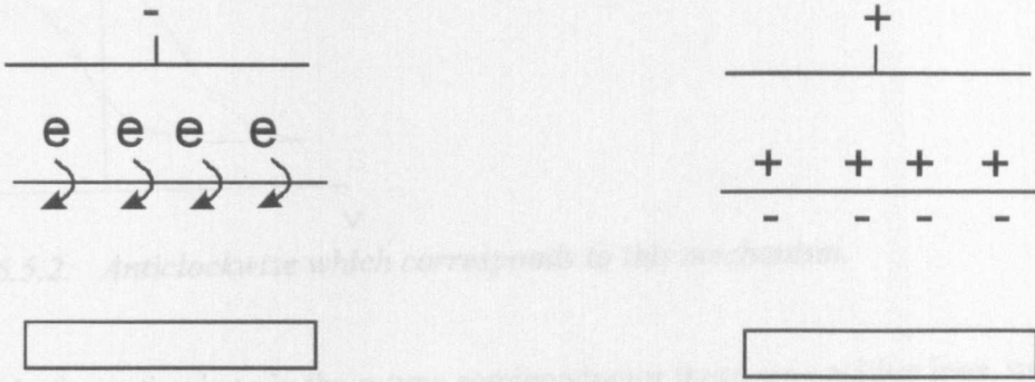
Figure 6.4.2(a): Electrons tunnelling from the dielectric to the semiconductor.
