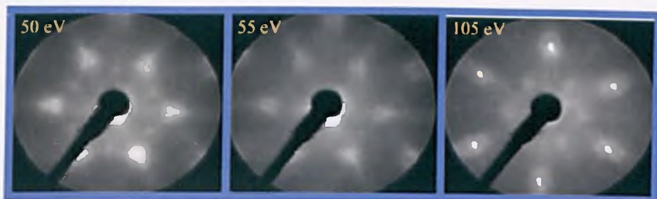
Figure 4.8: LEED pattern from a dissociated D_2O monolayer on Ru (0001) after extended electron exposure.
