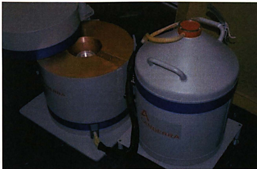
Figure 3.2 Photograph showing the Ultralow-level Canberra BE50 detector used for samples OR14, BLA1 and BLA3. The electrolytic copper on the inside of the detector can also be seen (Photograph courtesy of Dr Uwe Reiser, Victoria University of Wellington, New Zealand).
