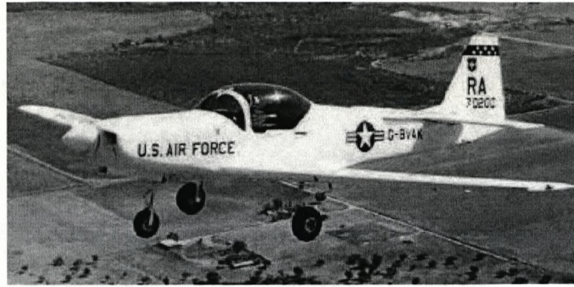
Figure 2.3. The first Slingsby model T67B made of composite materials [23].
