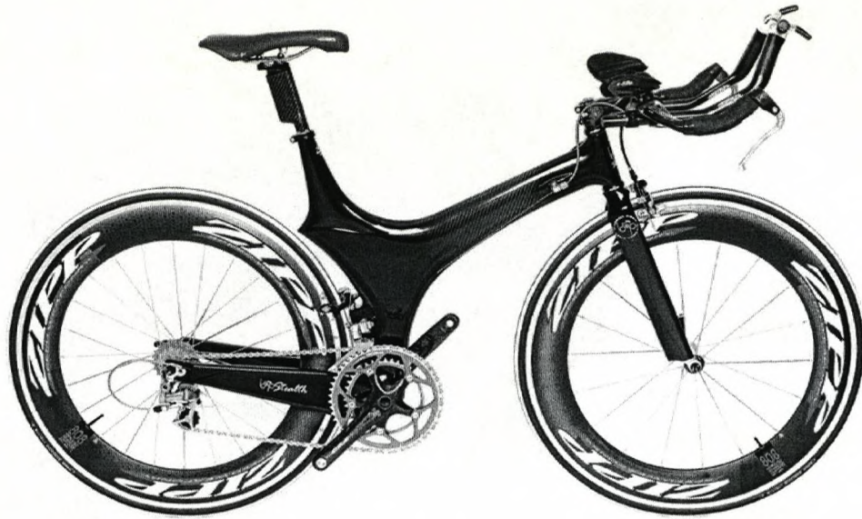
Figure 1.10. Lightweight bike with its all-composite frame [31].
