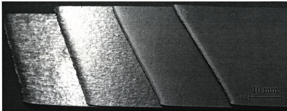
Figure 4.26. Photograph showing the four scaled aluminium coupons following tensile testing. From right to left, thicknesses of 0.5, 1.0, 1.6 and 2 mm.
