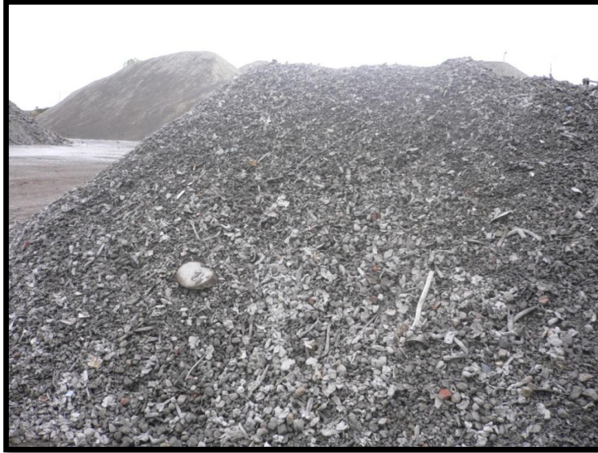
Figure 2-6: IBA stockpile before processing (Billingham, Teesside, UK).
