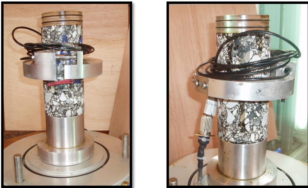
Figure 7-3: Sample instrumentation in the triaxial cell.
