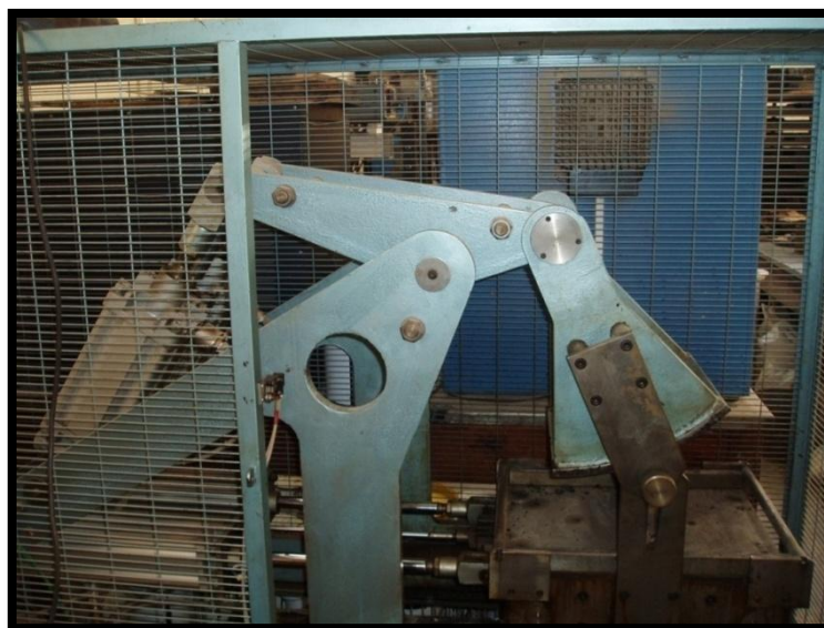
Figure 3-12: The laboratory roller compactor.
