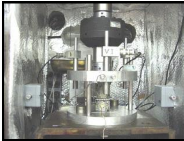
Figure 6-6: Radial strain measuring system used at TU Delft (Muraya 2007).
