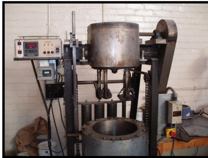
Figure 3-11: The laboratory asphalt mixture.
