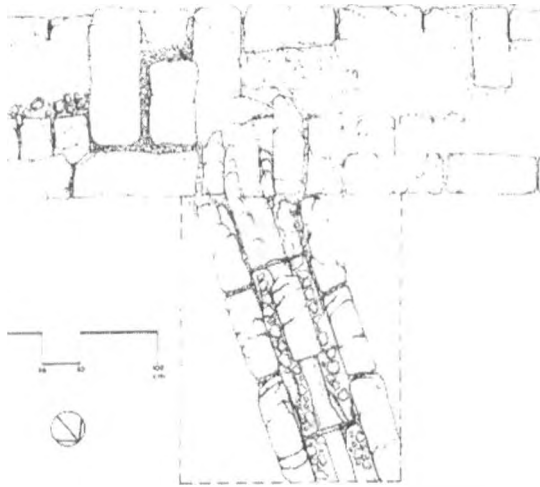
Fig. 3.41 Junction of the aqueduct and Cistern 2 at Humayma (Eadie & Oleson 1986: 60).
