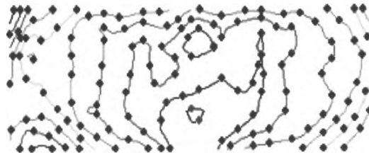
Figure 5.3.19: Irradiation strategy for pass 5
