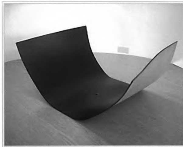
Figure 5.2.21: Highly formed component using the original irradiation pattern from pass 1
