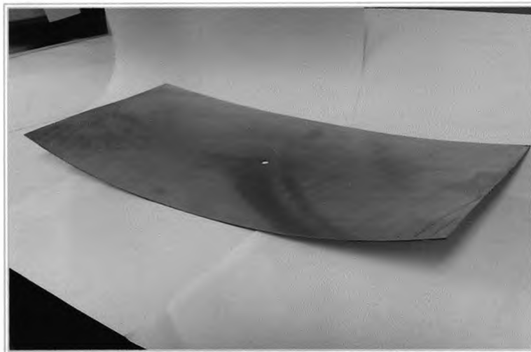
Figure 5.3.44: Picture of final shape 400x200x1mm AA5251, 200W, 3mm beam diameter, speed 29mm/s.
