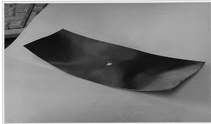
Figure 5.3.36: Picture of final shape 200x80x1mm AA5251, 200W, 3mm beam diameter, speed range 25-32mm/s.
