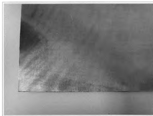
Figure 5.3.37: Marks from the 3D forming of 200x80x1mm AA5251 at 200W and a speed range of 25-32mm/s
