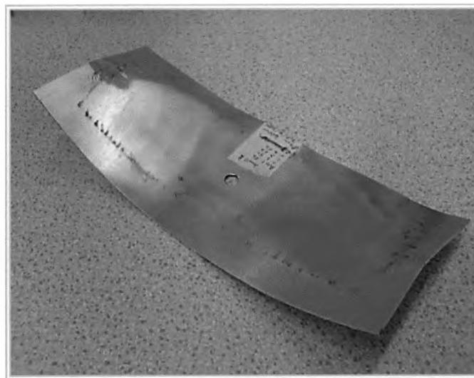
Figure 5.3.22: Heavily faceted component resulting from the initial strategy chosen
