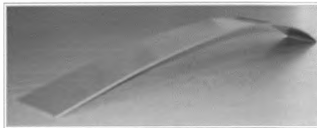
Figure 5.3.65: Strut with maximum 45mm mechanical deformation
