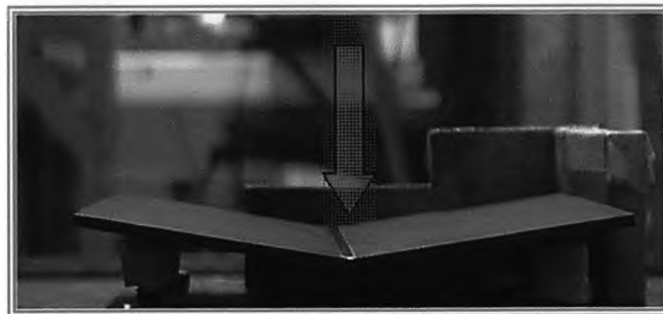
Figure 4.1.14: V-block or simply supported clamping arrangement.
