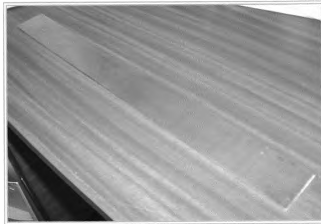
Figure 5.3.66: Strut after laser forming correction
