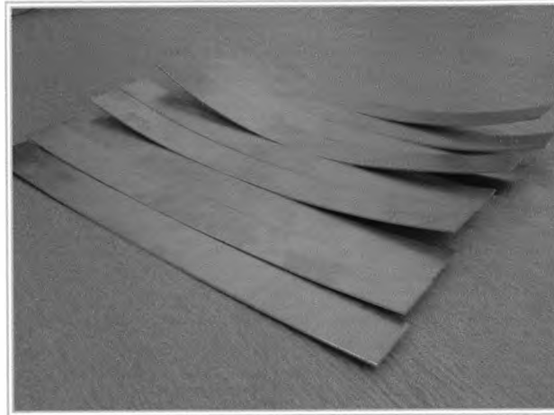
Figure 5.3.46: Randomly mechanically distorted components (400x40x2mm AA5251).
