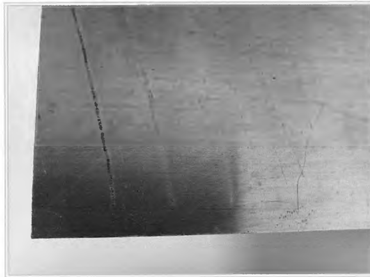
Figure 5.3.43: Marks from the 3D forming of 400x200x1mm AA5251 at 200W and a speed range of 31.4-35.9mm/s. The marks on the left are where the piece comes into the focus of the laser beam.
