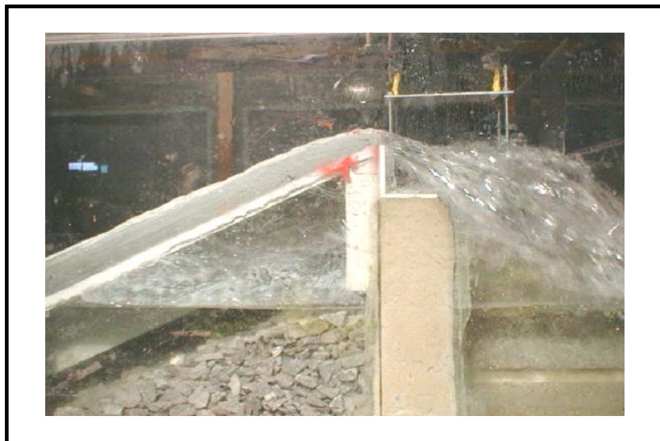
Figure 3-34 Snapshot of an overtopping event
