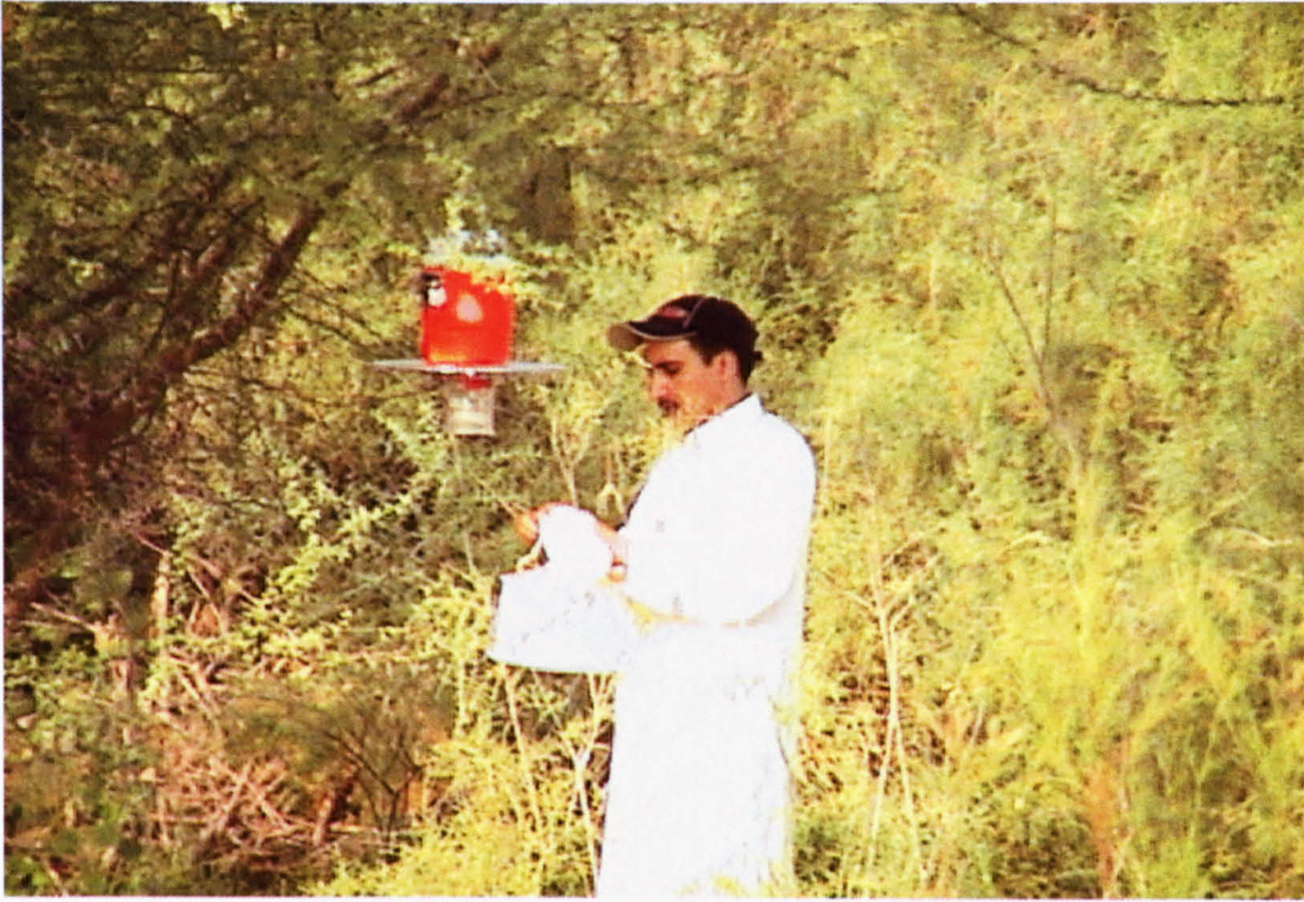
Figure 3.5: CDC light-traps baited with CO 2 used to sample outdoor mosquitoes in the Dam area, Rawan Alabeed, Jizan Region, Saudi Arabia.
