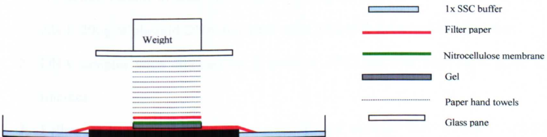
Figure 2.7.4 Set up of Southern blot transfer of DNA from gel to membrane
