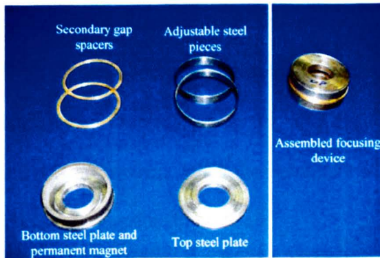
Figure 6.8. Picture of the magnet focusing device.
