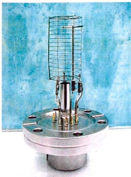
Figure 3.4. The B-A ionization gauge.
