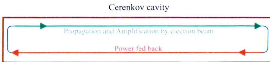
Figure 2.4. The feedback and amplification process of the FEL power.
