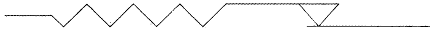
Figure 4.2.1 A linear spring and Coulomb friction element connected in series to create a Jenkins element.
