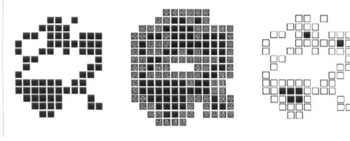
Figure 2.1: Original image (left), dilated (middle), eroded (right) by a 3 \times 3 square SE.
