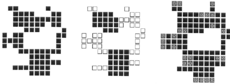
Figure 2.2: Original image, opening, closing by 3 \times 3 square.
