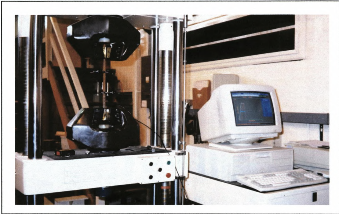
Figure 5.5 Denison universal test rig is testing tensile of steel reinforcement
