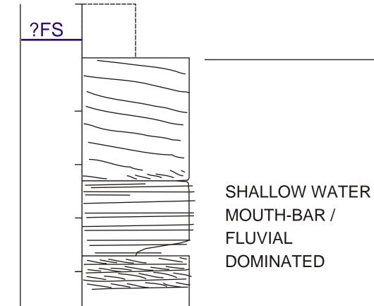
dominated by current ripple laminated sandstone, with some parallel bedded, suspension deposited sand, upper 2m may represent depsitional dip of proximal sand dominated mouth-bar
