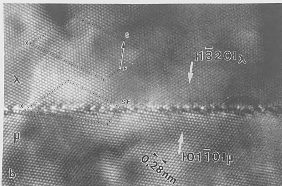
Fig 6.2: High-resolution micrograph of 17.8° tilt boundary. After ref [1]
