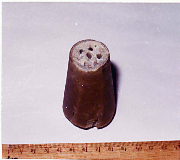
Figure 4.4. Strand II. Resin cone after wires pulled out.
