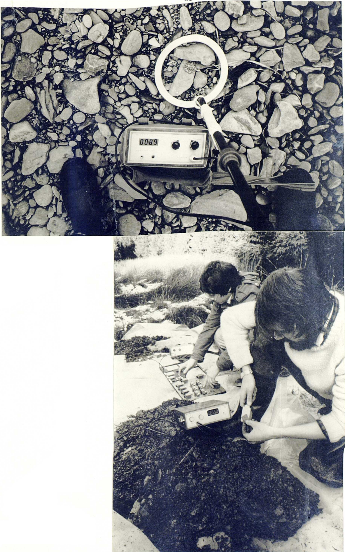
PLATE 3.1. FIELD INSTRUMENTATION FOR MEASURING MAGNETIC SUSCEPTIBILITY SHOWING CONTROL UNIT AND DIGITAL OUTPUT, SEARCH LOOP AND FERRITE PROBE.
