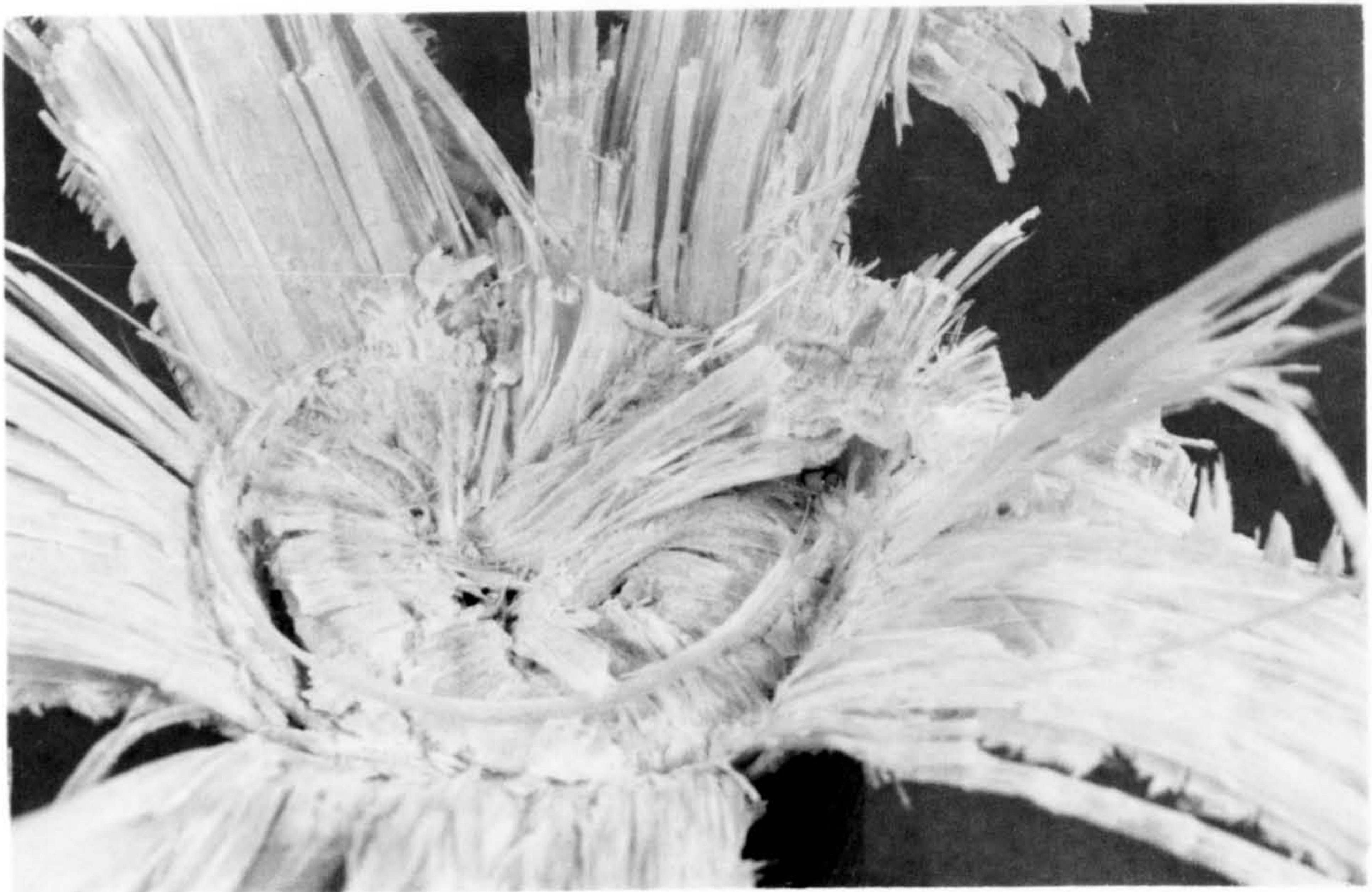
(b) Close-up of crush zone. Axial fibres break and bend inwards and outwards.
