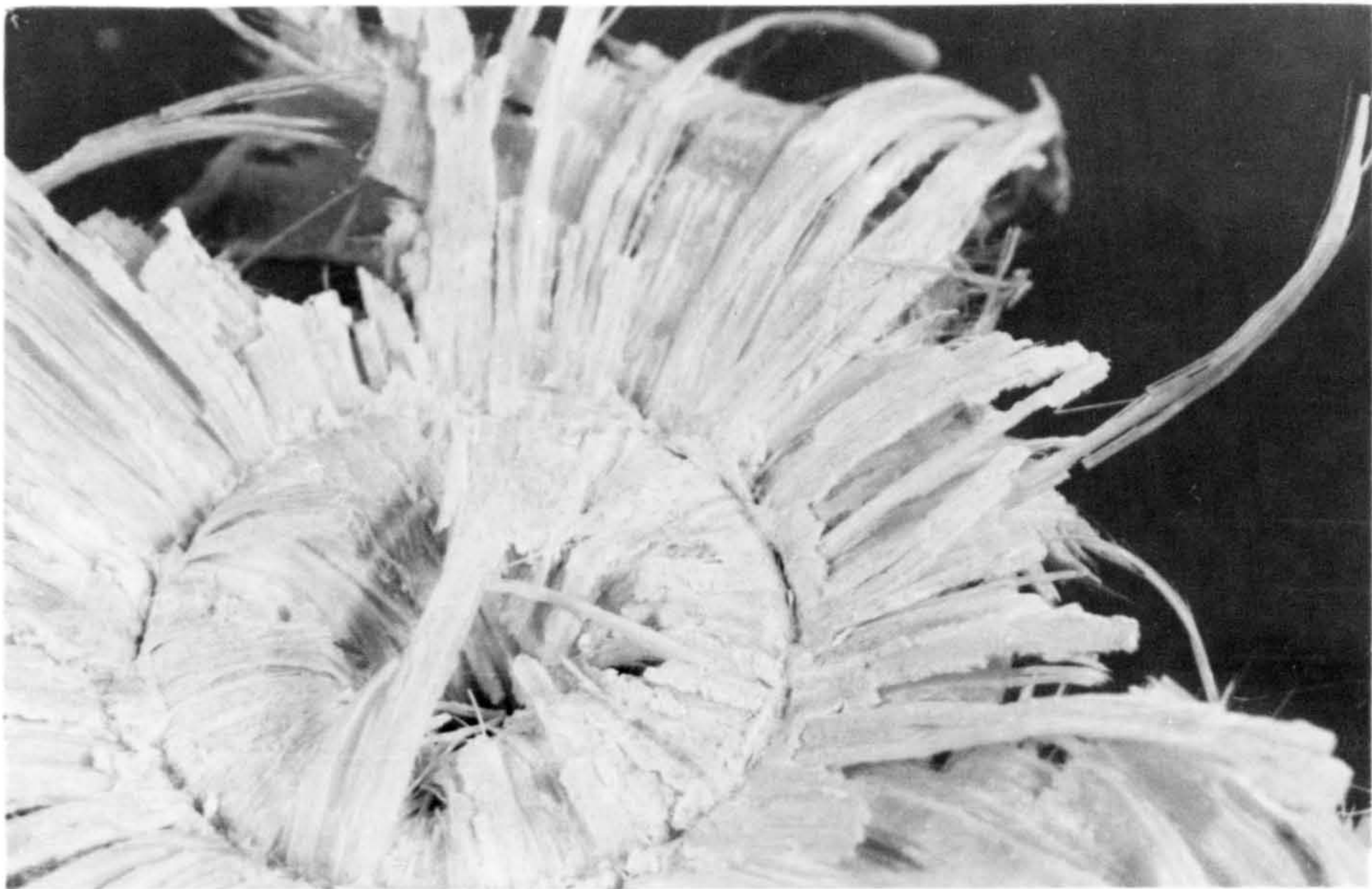
(b) Close-up of crush zone showing fractured fibres.
