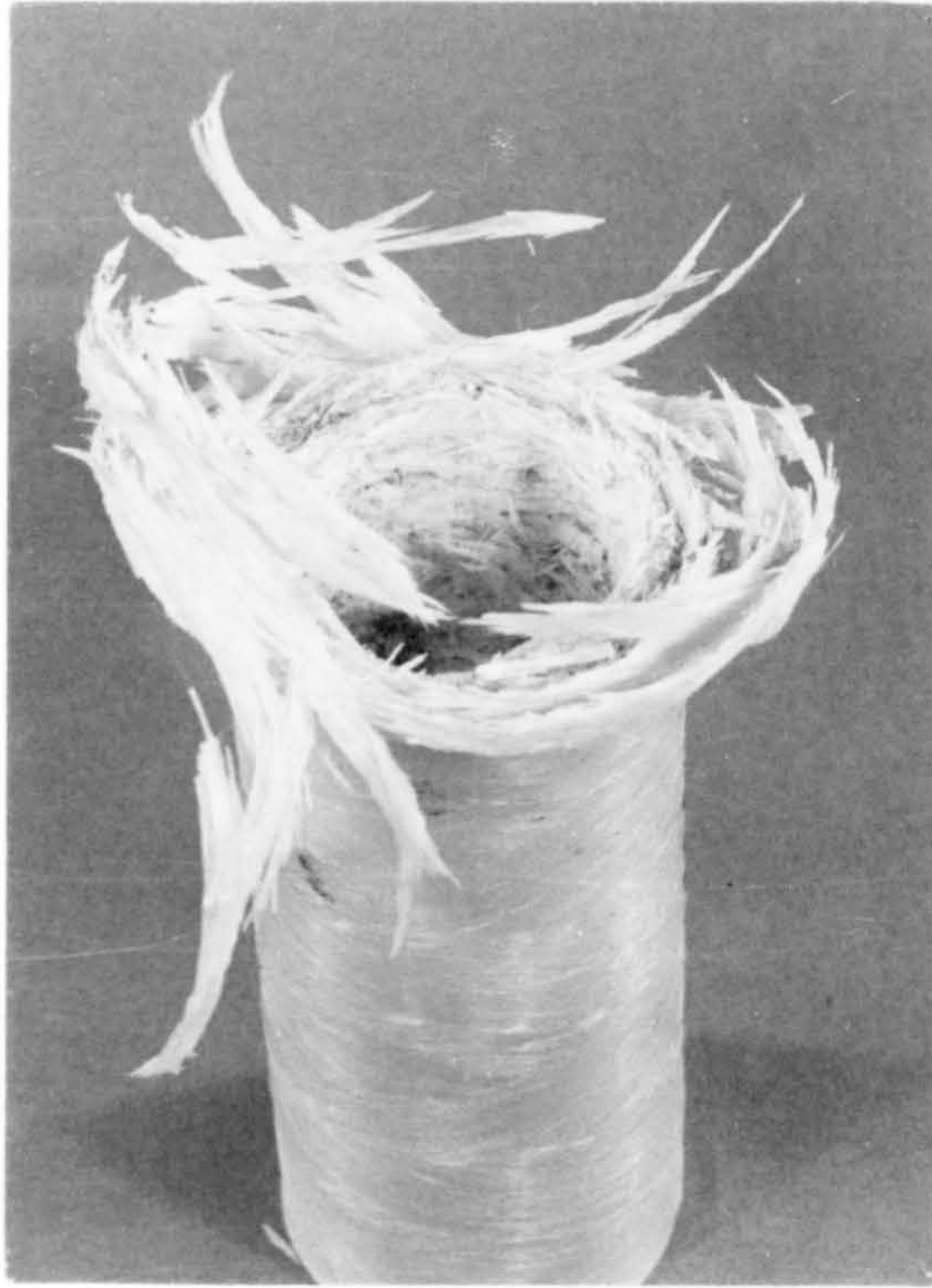
(a) General view of crush zone.
