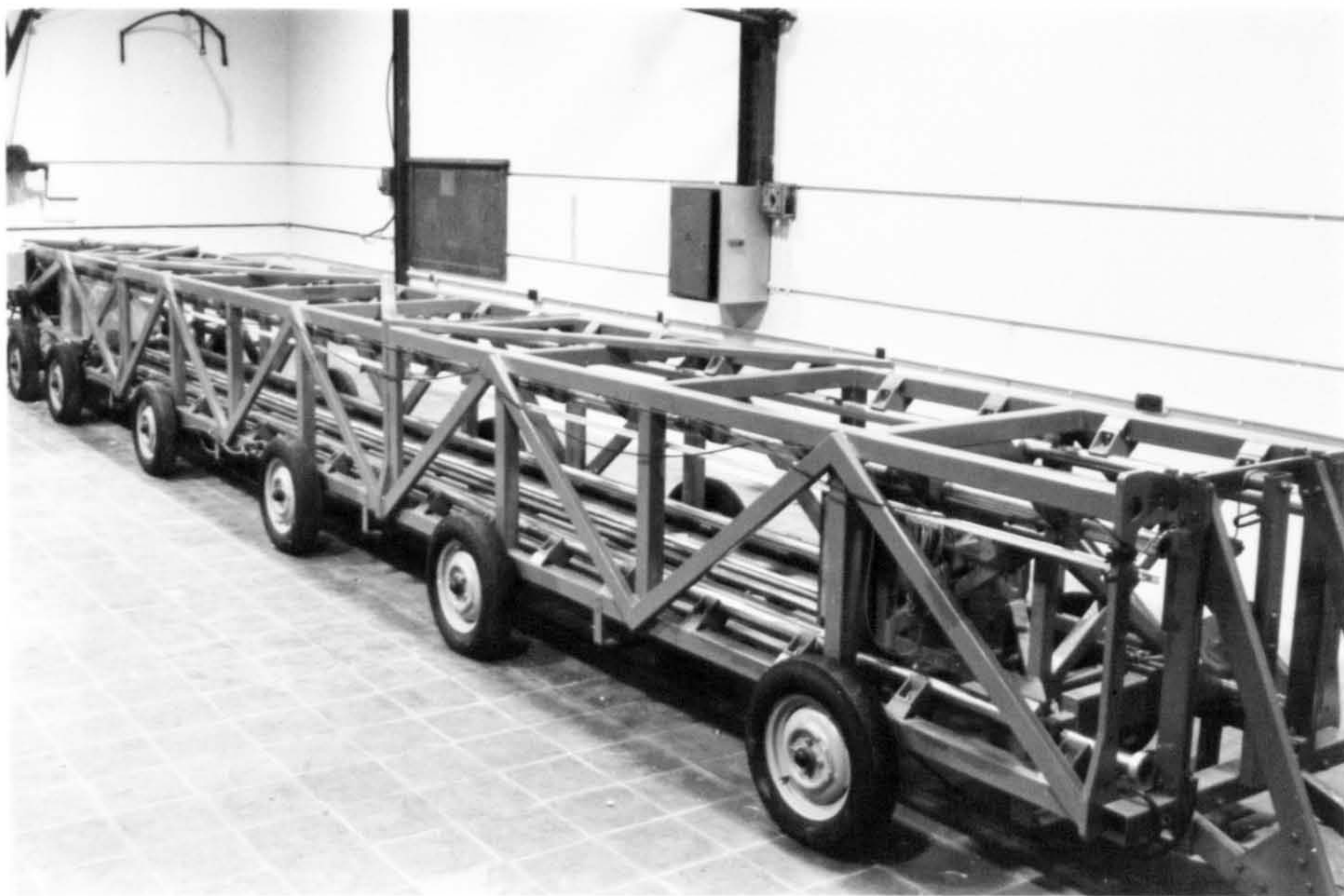
Fig.3.6. Photograph of the crash rig.Target plate is at the far end.
