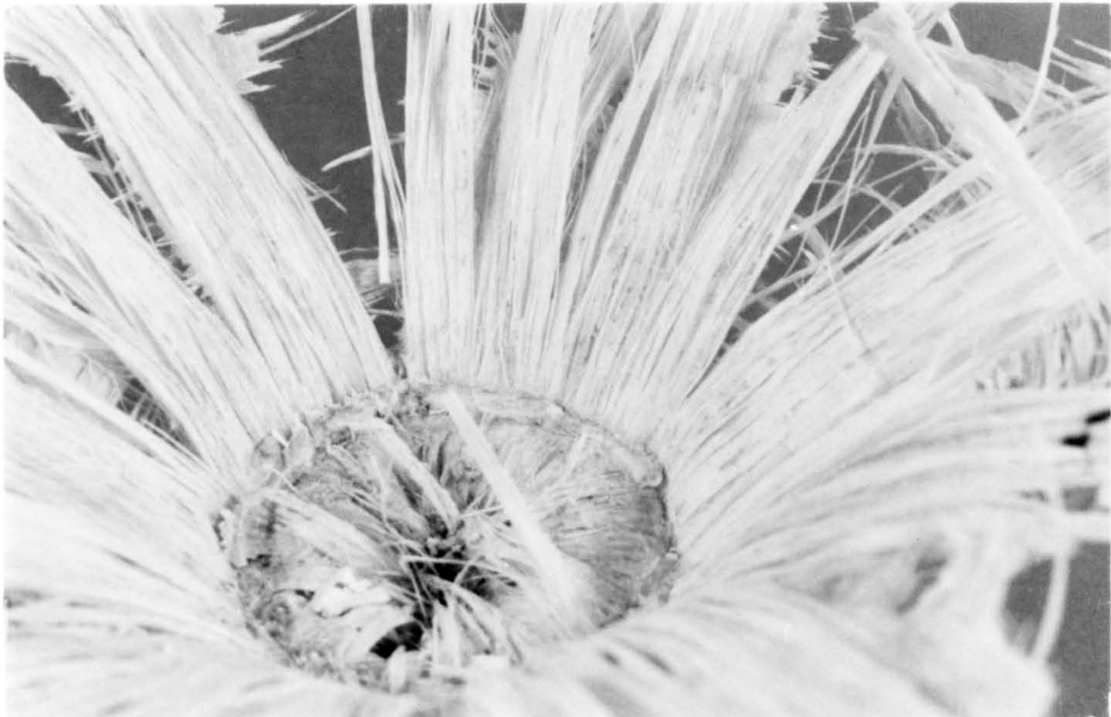
(b) Close-up of crush zone. Axial fibres bend inwards and outwards. Outer axial fibres are generally unbroken.
