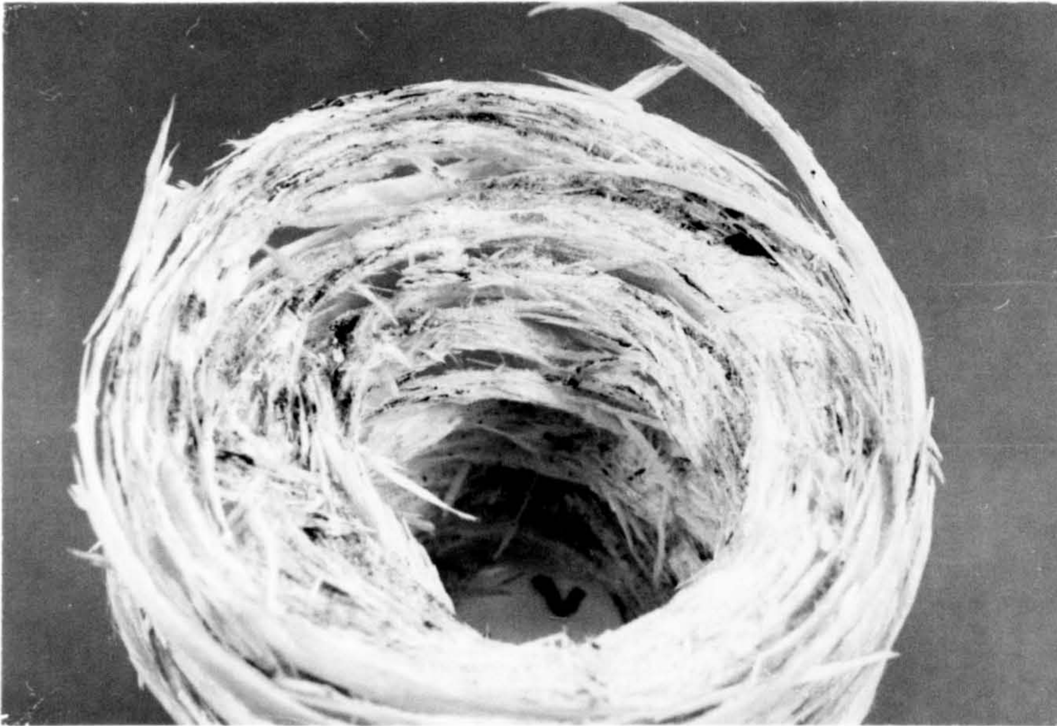
(b) Close-up of crush zone showing long fibre tows detached from the tube wall.
