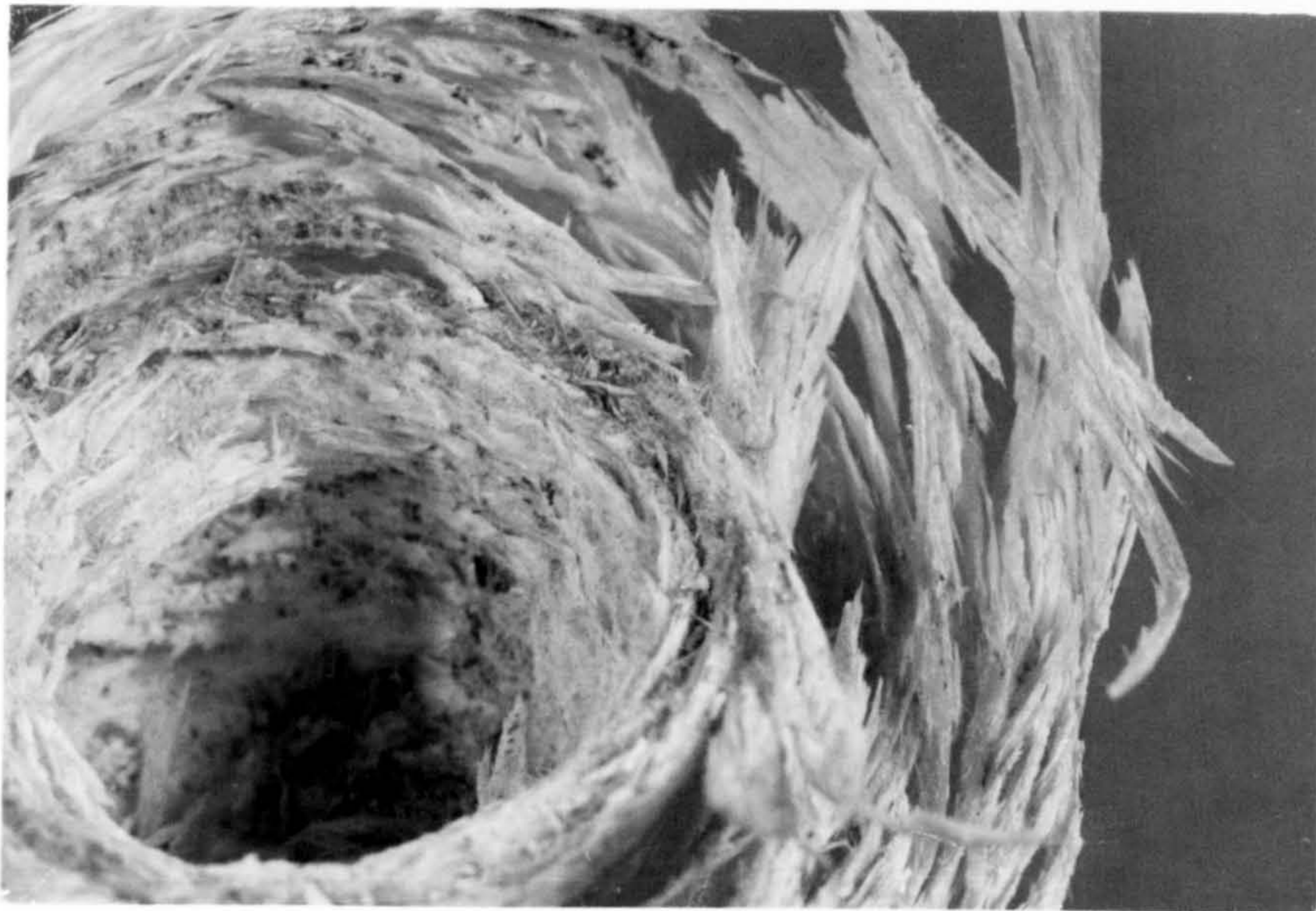
(b) Close-up of crush zone showing long detached fibre tows.
