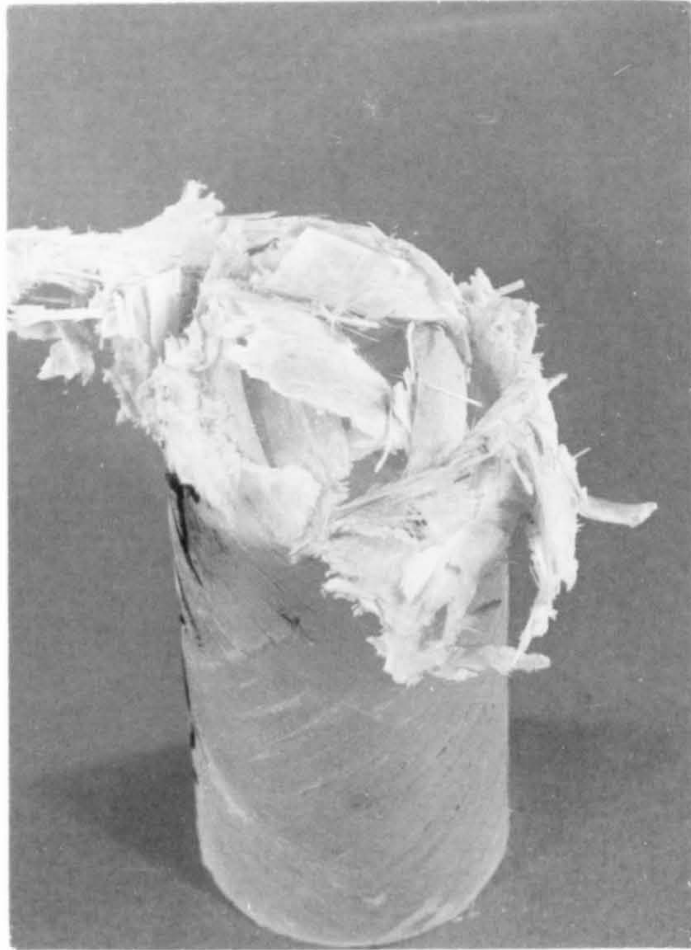
(a) General view of crush zone.
