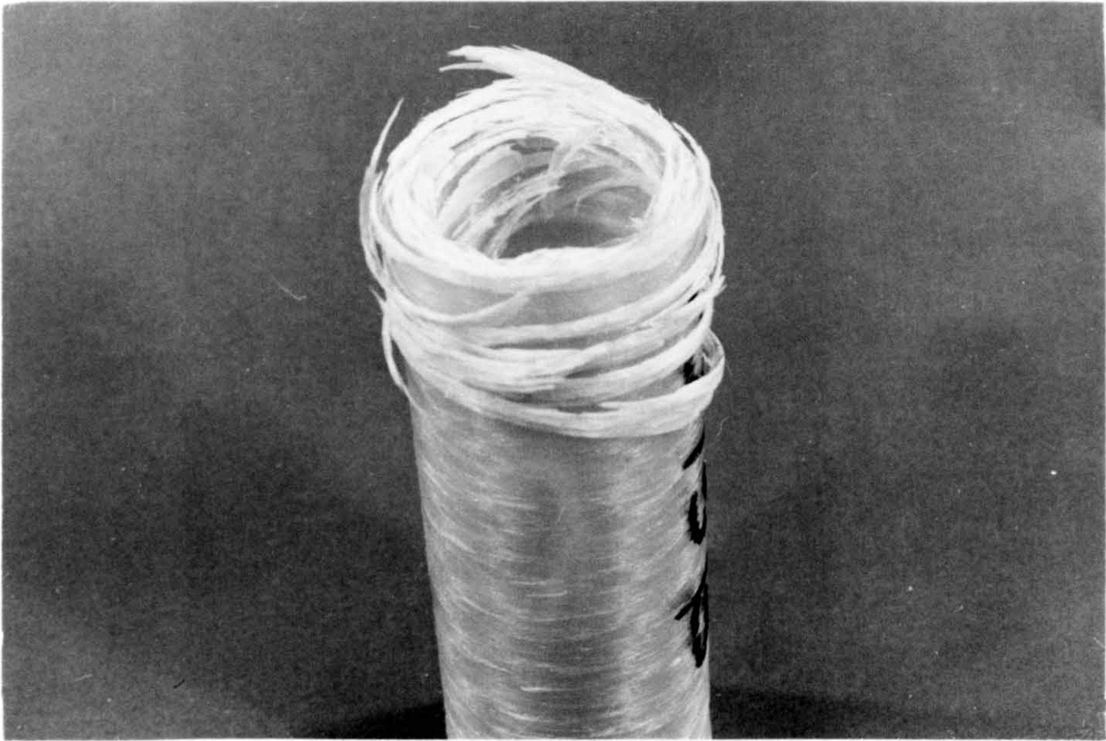
(a) General view of crush zone.
