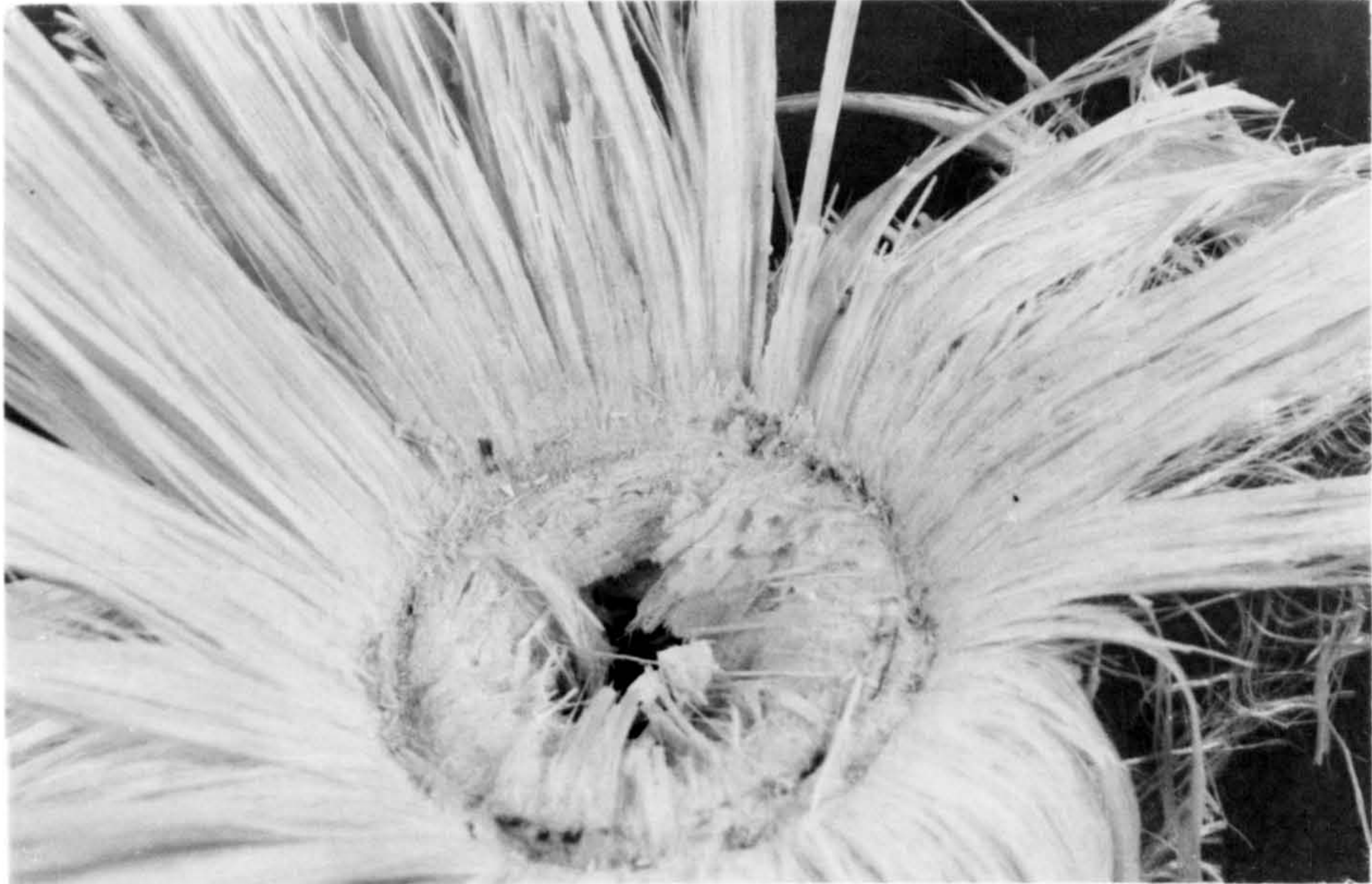
(b) Close-up of crush zone showing unbroken axial fibres.
