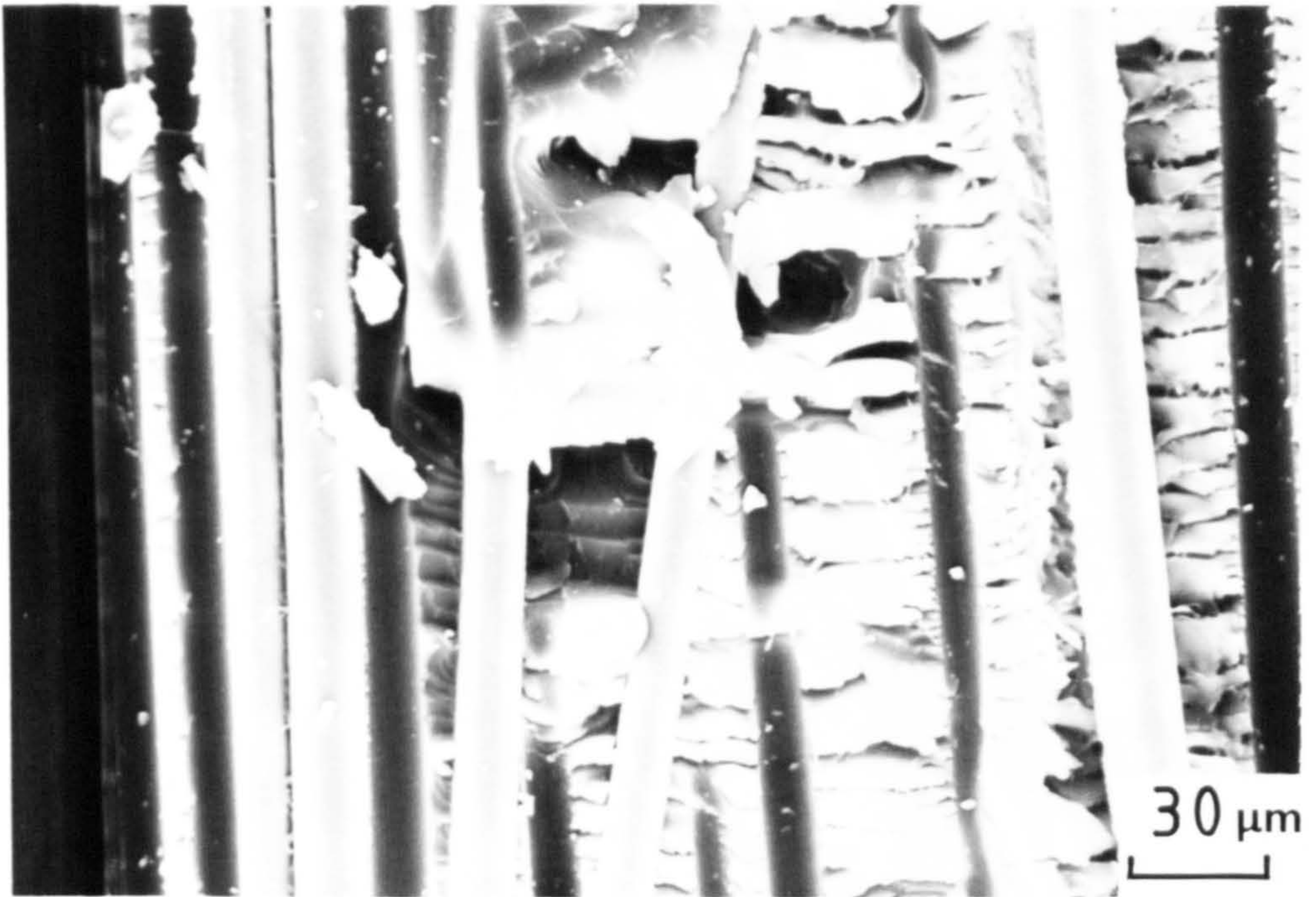
(a) Fracture surface showing clean fibres with jagged torn resin.
