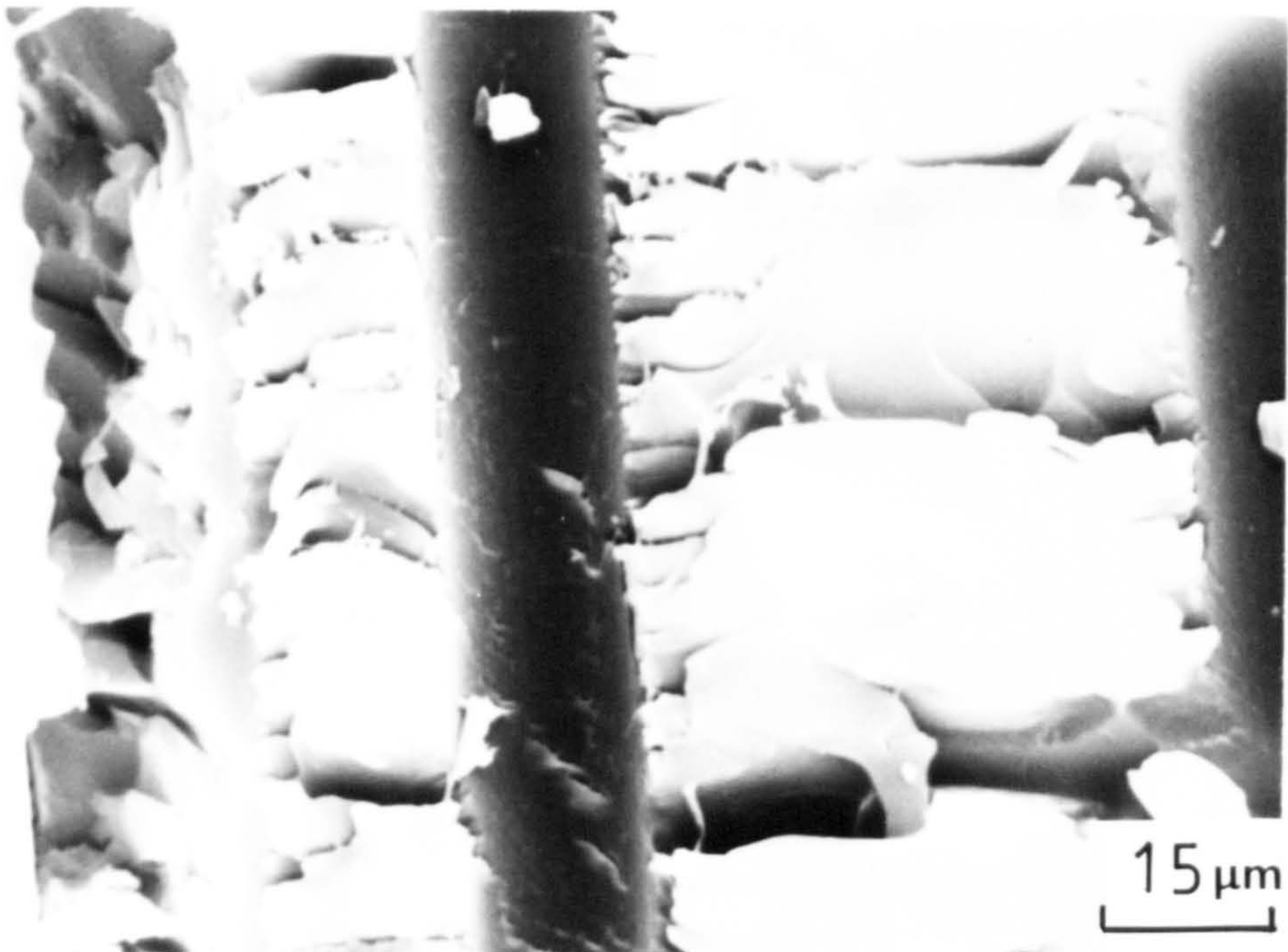
(b) Higher magnification showing resin fracture surface.
