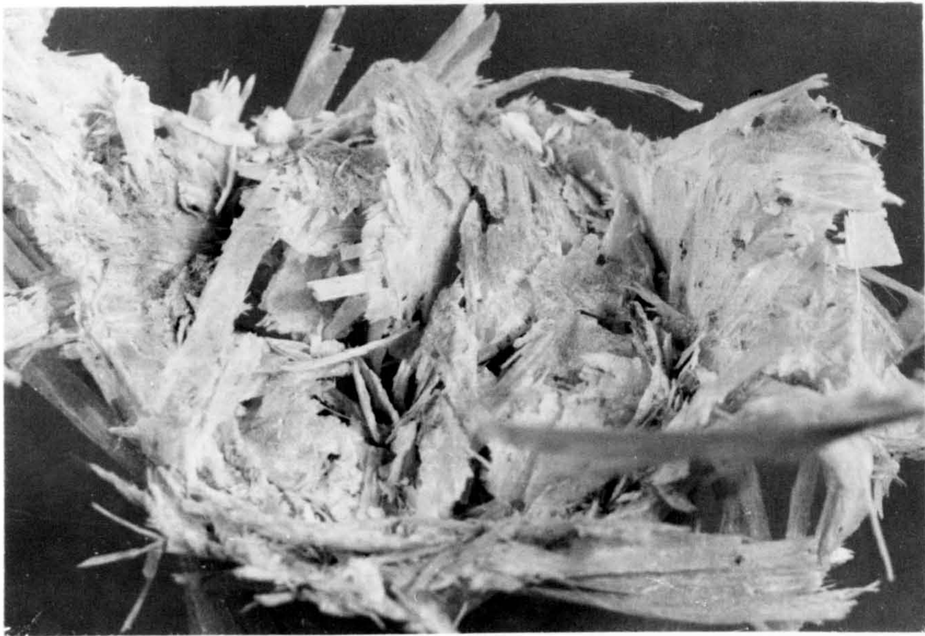
(b) Close-up of crush zone. Lamina plates bend inwards and outwards.
