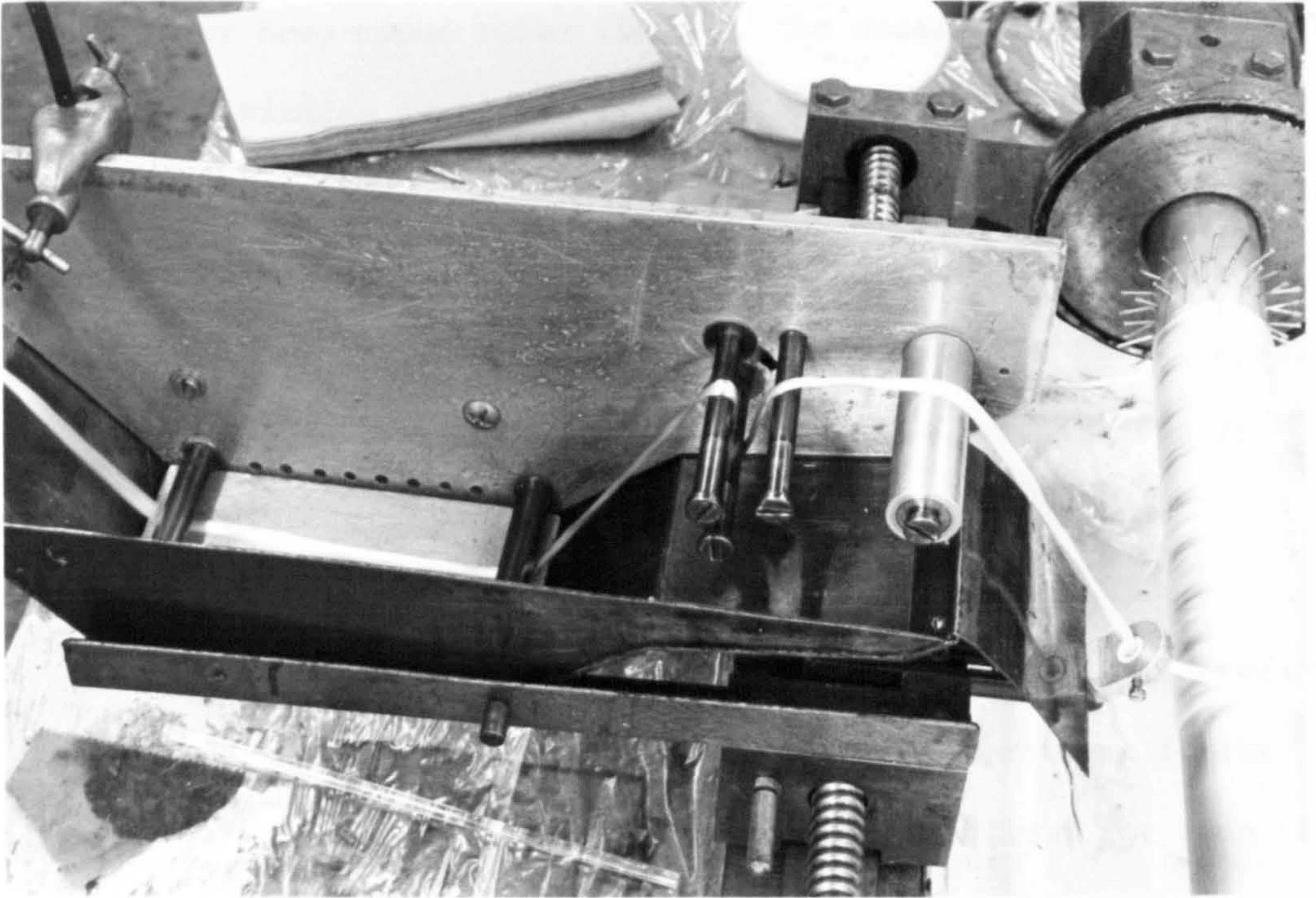
Fig.3.2. Resin bath on the filament winding machine. Note the glass fibres passing through the bath and around the guide pins. Resin omitted to improve clarity.
