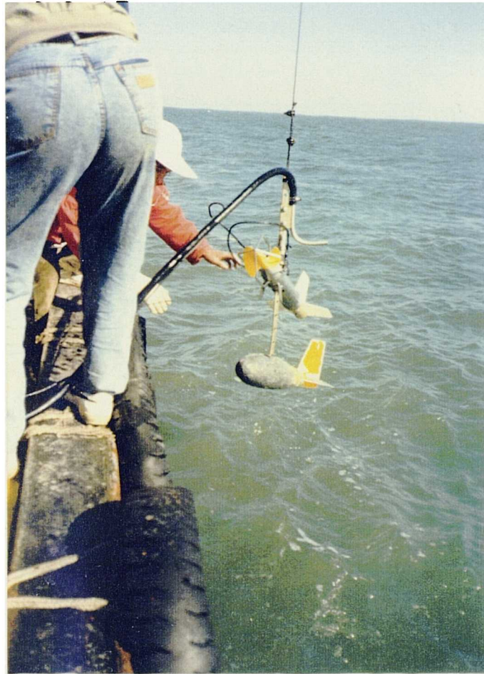
Plate 8.2a HR suspended sediment pump sampler used for measuring suspended sediment concentration: intake pipe.
