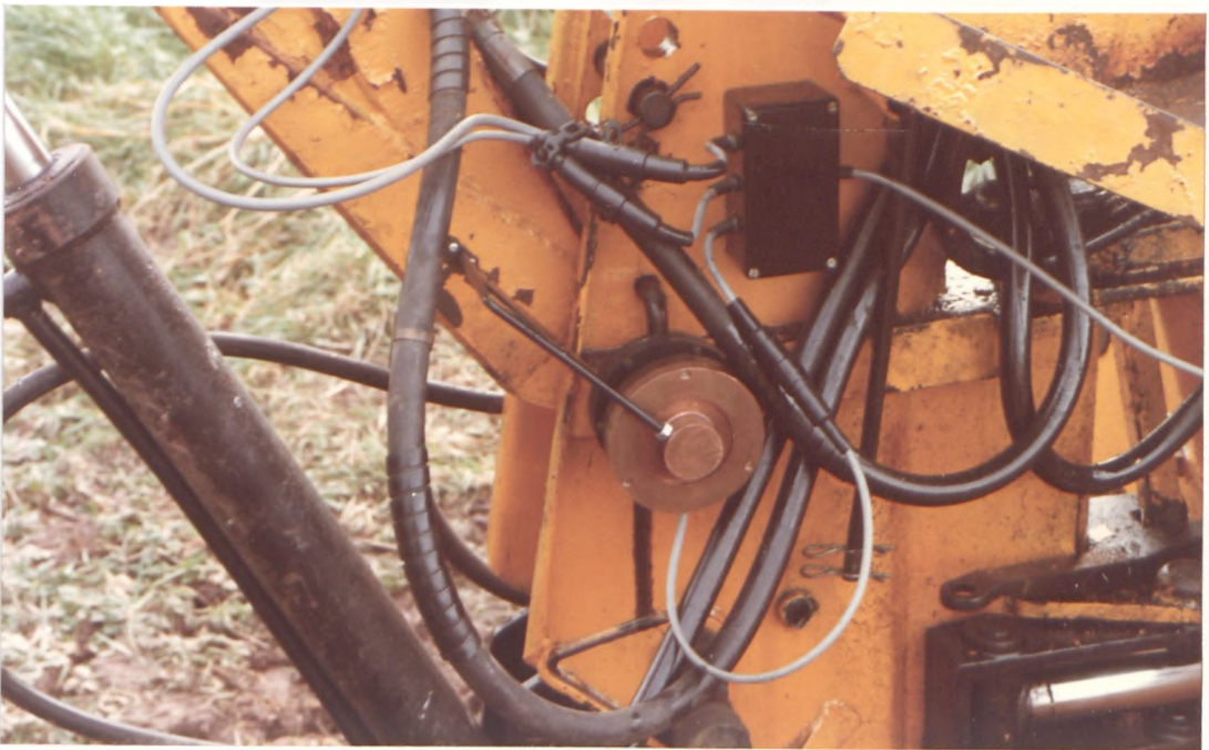
Plate II : Lift Transducer showing Junction Box
