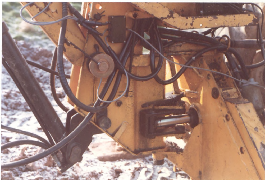
Plate XIII: Side View of Machine Showing Junction Box & Transducer for Main Arm
