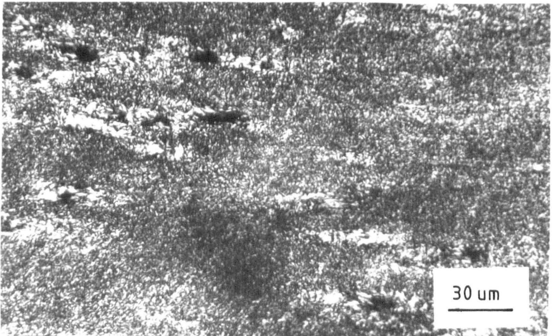
Figure 4.28. Optical transmitted light photograph of the reinforced polymer, 2.0mm section at the centre of the moulding, layer IV, parallel to the flow direction. Magnification = 560.
