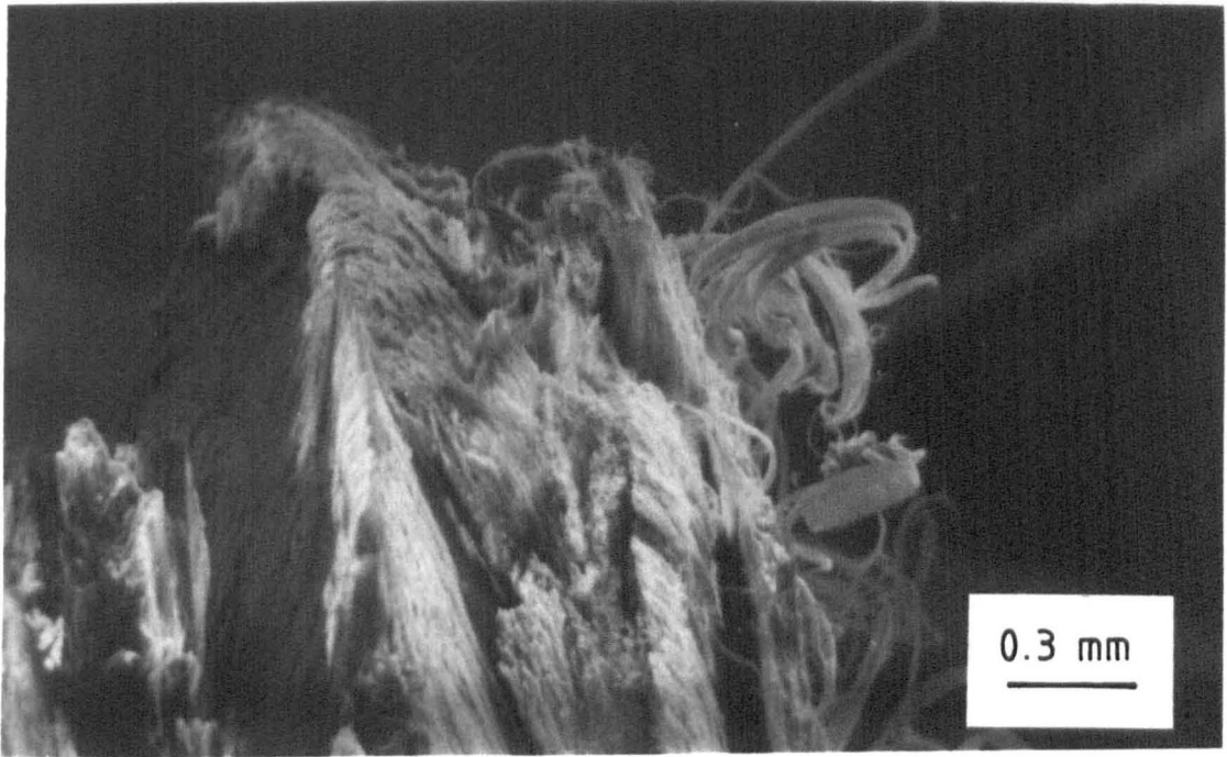
Figure 4.33. Scanning electron micrograph of a fracture surface for the unreinforced polymer, 2.0mm section, tested in tension, parallel to the flow direction. Magnification = 50.
