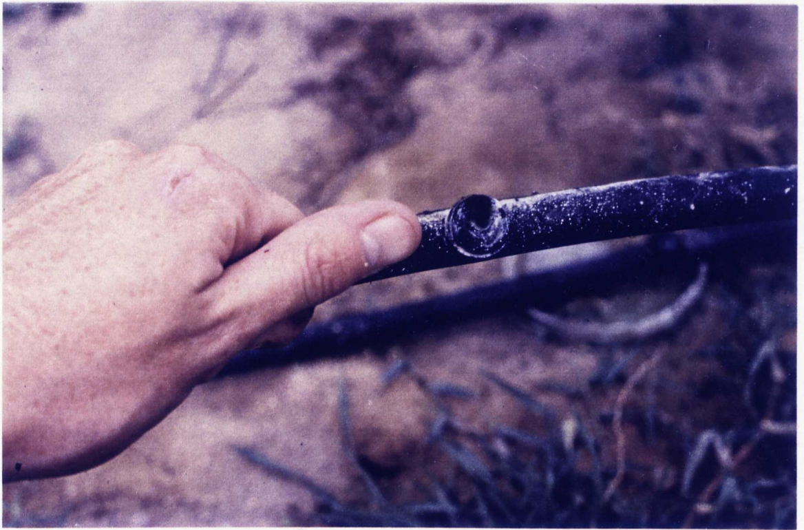
Plate 5.4 An example of Emitter C in operation showing a cyanobacterial mat and calcium carbonate precipitation
