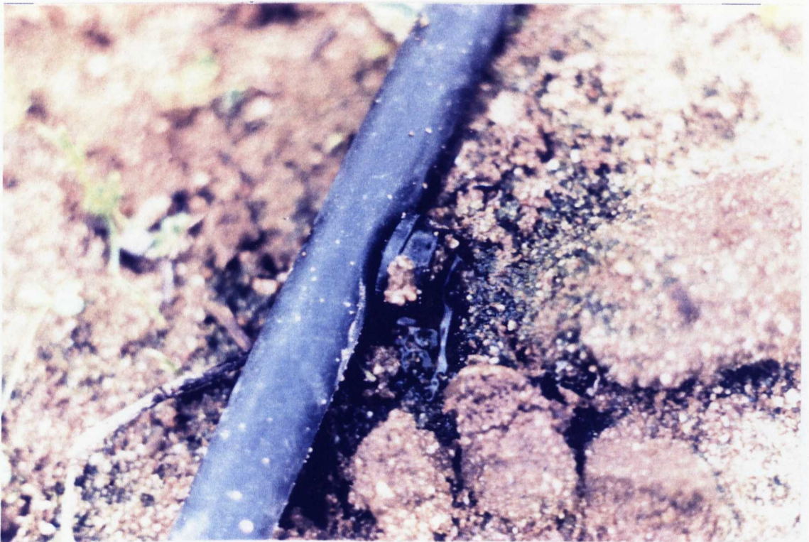
Plate 5.5 Growth of filamentous cyanobacteria on the soil surrounding an emitter discharging WSP effluent
