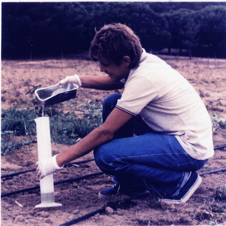
Plate 2.6 Measuring emitter output
