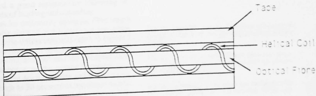
Stress-responsive intrinsic fibre sensors: Fig 2a (above), speckle pattern; and Fig 2b (below), microbending helix.
