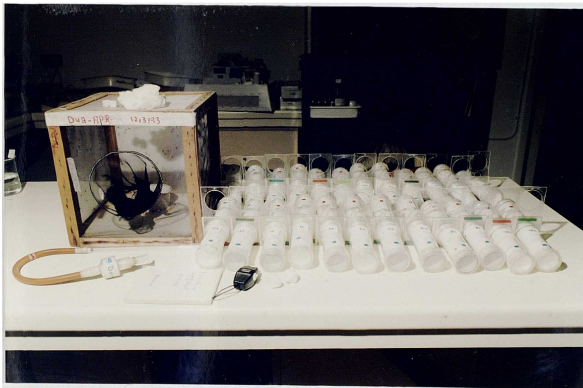
Fig. 3.3 Insecticide testing method for adults according to WHO (1970) with some modification
