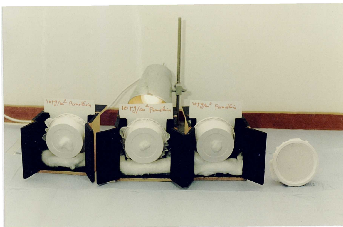
Fig. 3.8 Modified insecticide irritability chamber used for testing vapour effect
