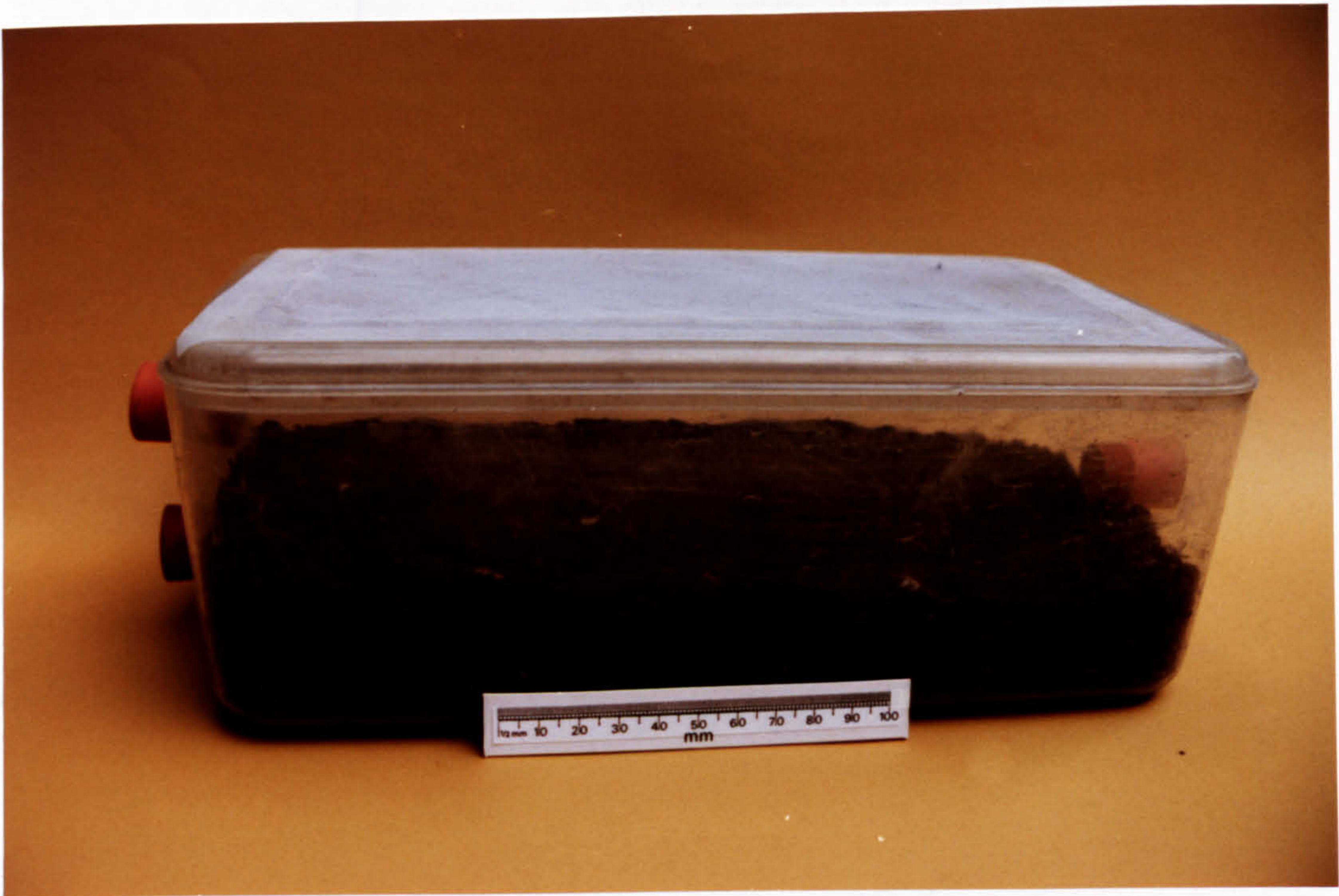
Figure 2.3 Control container for temperature and humidity measurements showing position of rubber bungs where temperature/humidity probe was inserted.
