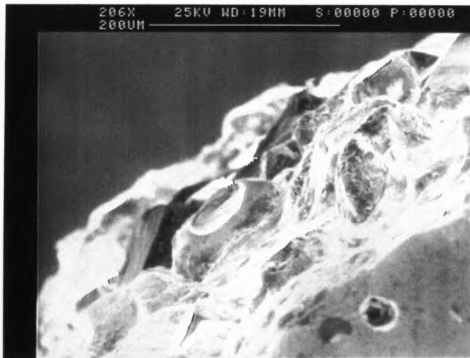
Fig. 7.16 SiC particles covering clad surface (upper) and embedded in upper part of clad (lower)
