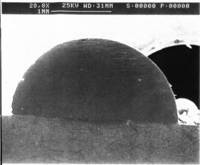
Scanning electron micrograph showing dimensions of a typical clad
