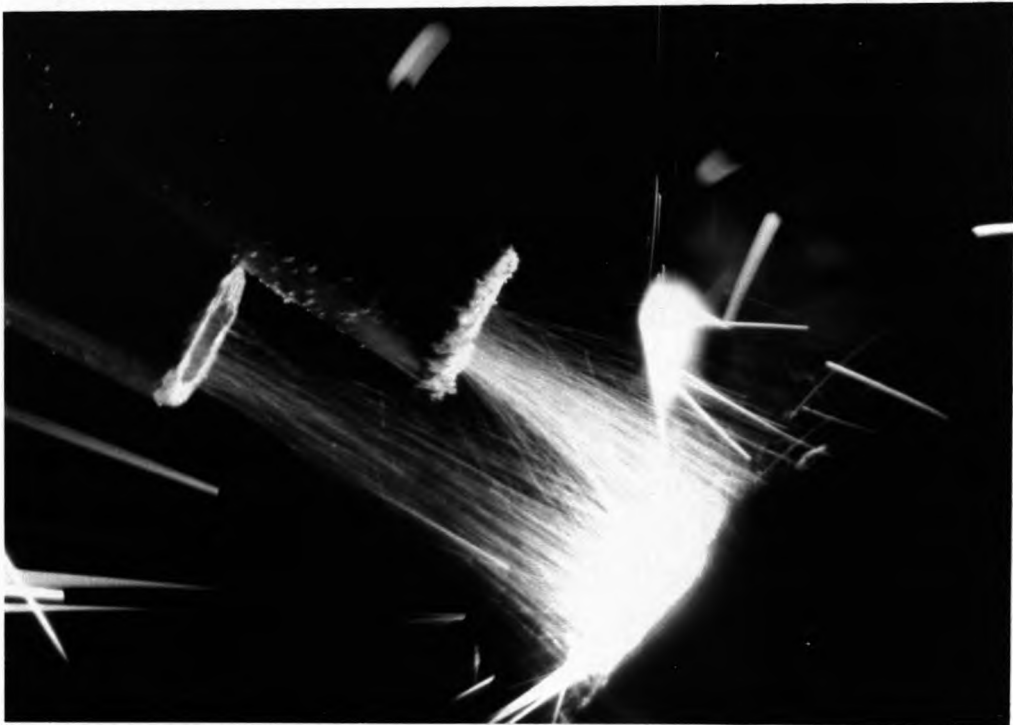
Fig. 7.20 Two geometries used for cladding of Stellite 35 and ceramic powders
