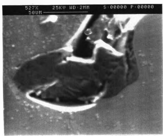
Scanning electron micrograph of undissolved SiC particle, near surface
