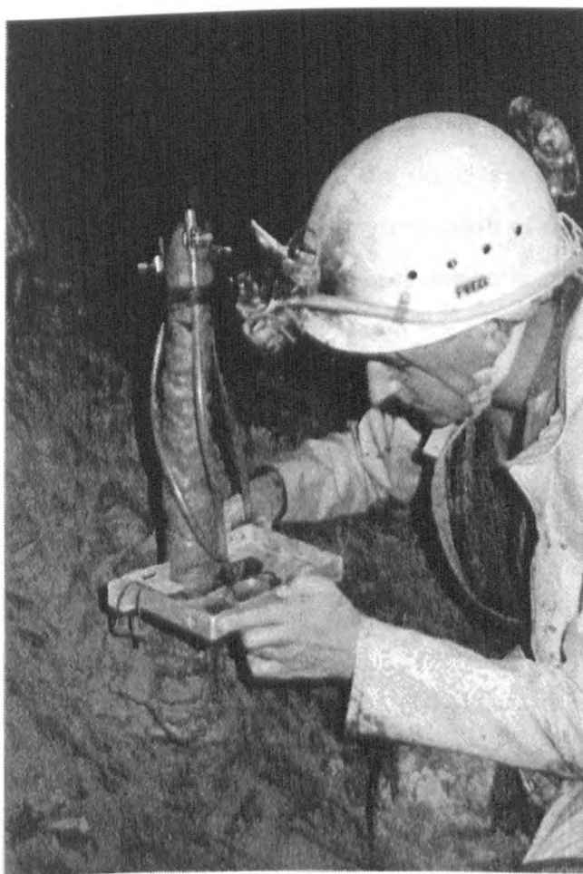
Photograph 5.1. Orienting stalagmite TR01 in the cave using the 3-Arm U-tube and aluminium frame.
