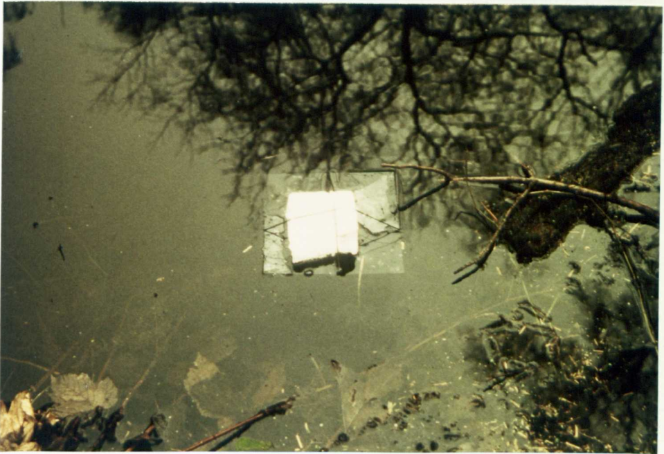
Fig. 15: A floating sticky trap in a ditch. The adhesive is coated on the undersurface of the transparent plastic sheet which is then floated on the water by a piece of polystyrene.
