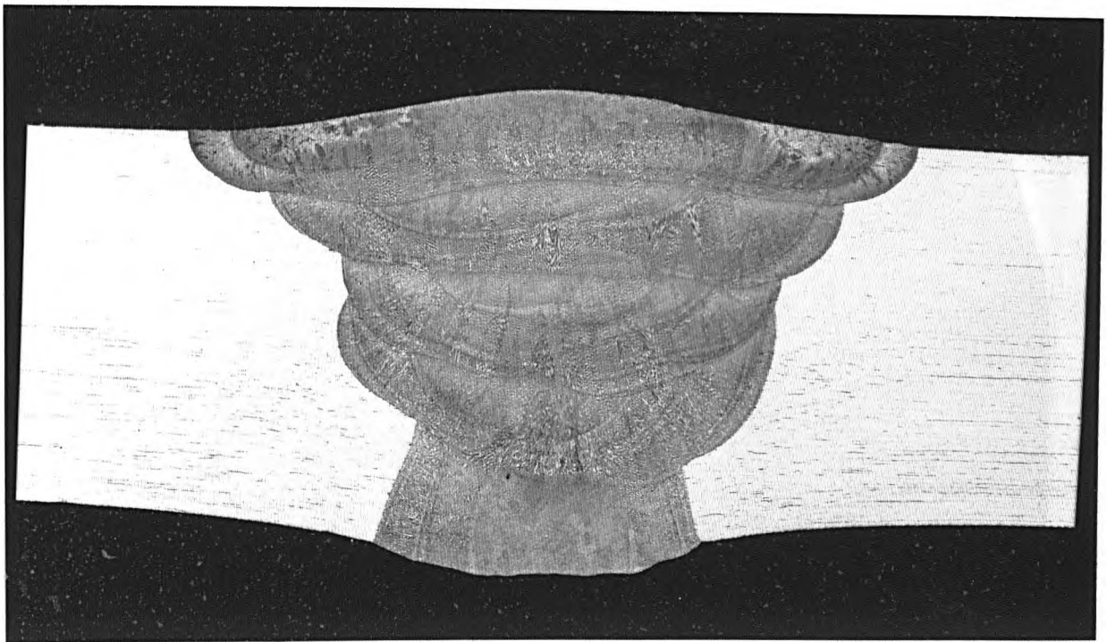
(b) Cross section of weld
