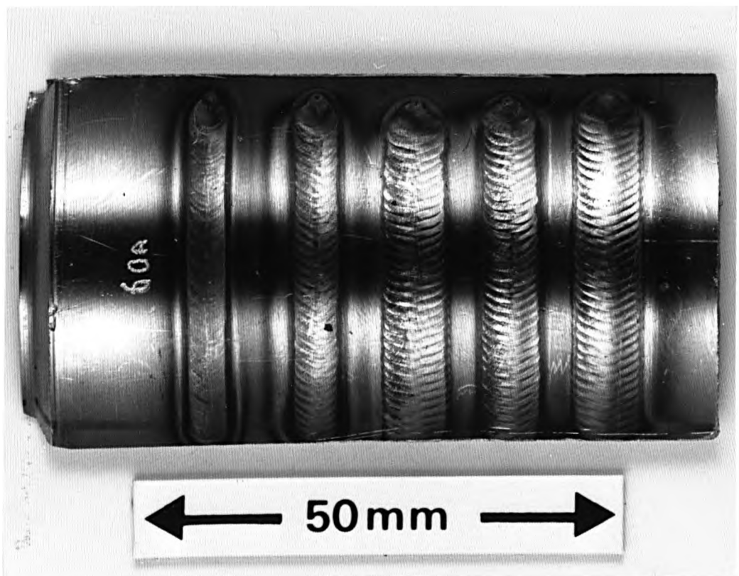
(b) Welding current: 60A
