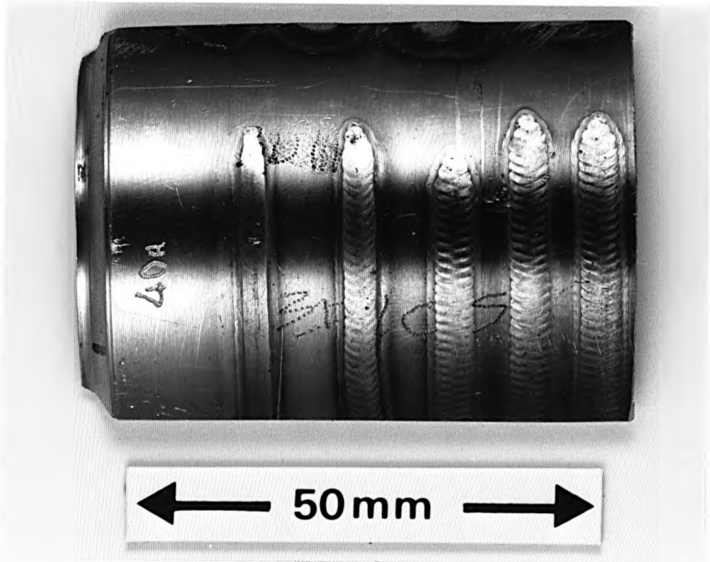
(a) Welding current: 40A
