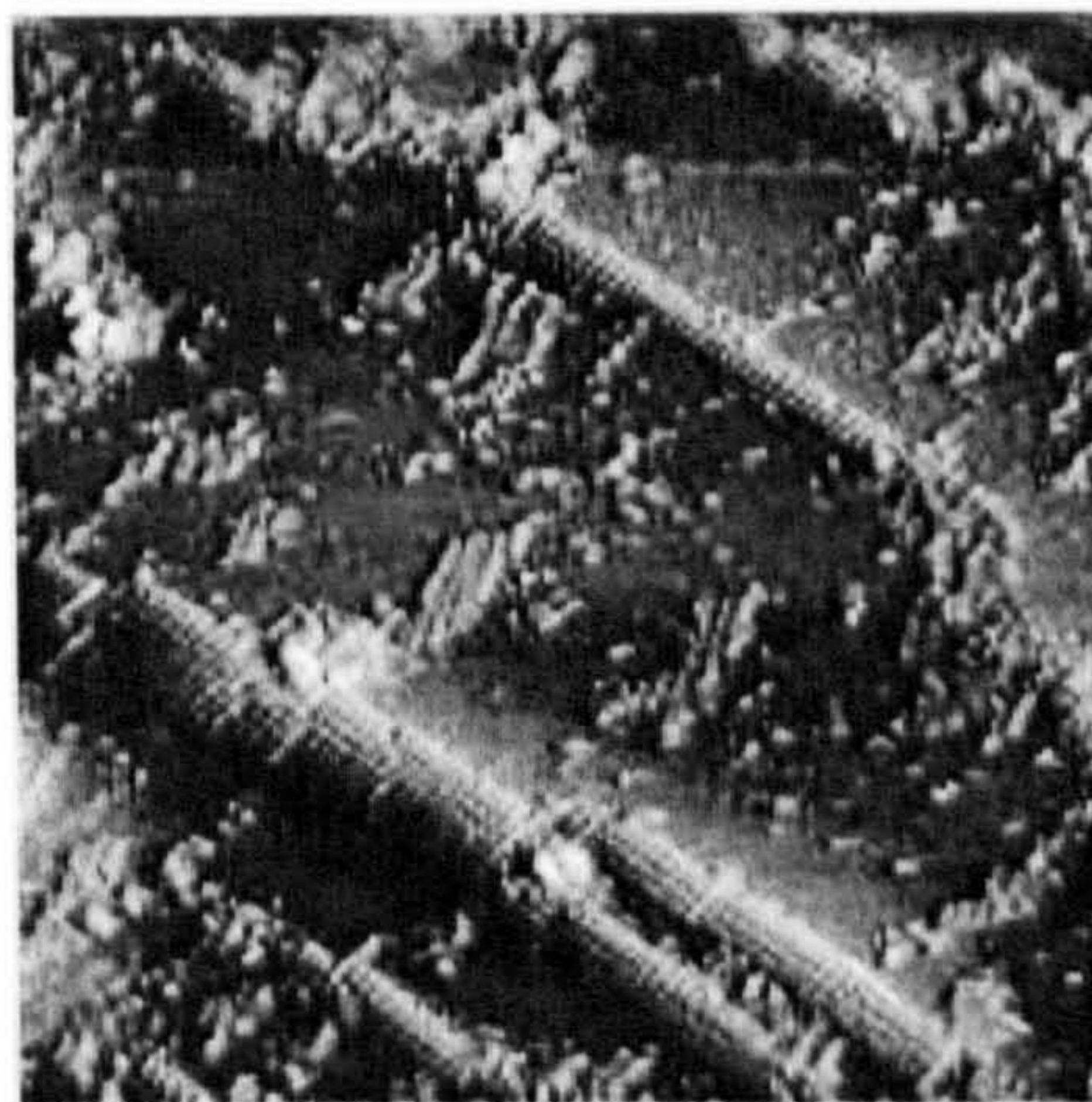
Figure 5.10: STM image representing the “low coverage” of (S)-alanine adsorbed on the Cu (110) surface, 500 \text{ \AA} \times 500 \text{ \AA} [10].
