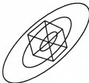
Figure 23. The simplex reaches the best response for a system and circulates around the optimum response. Further application of the simplex rules in such a situation only serves to cause the simplex to circulate around the best response. 206
