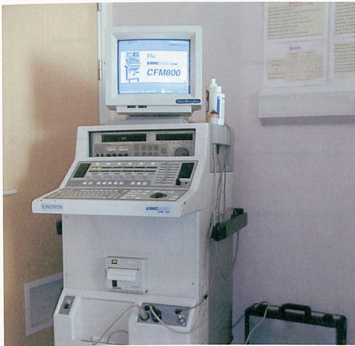
Figure 2.2: General Electric Colour Flow Mapping 800 series, incorporating a multifrequency 5 to 7.5 MHz imaging transducer, colour flow mapping, high frequency pulse wave Doppler and continuous wave Doppler and an integrated digital archiving system, an Apple Macintosh computer using the Echopac software version 5.3 (General Electric Ultrasound, Bedford UK).
