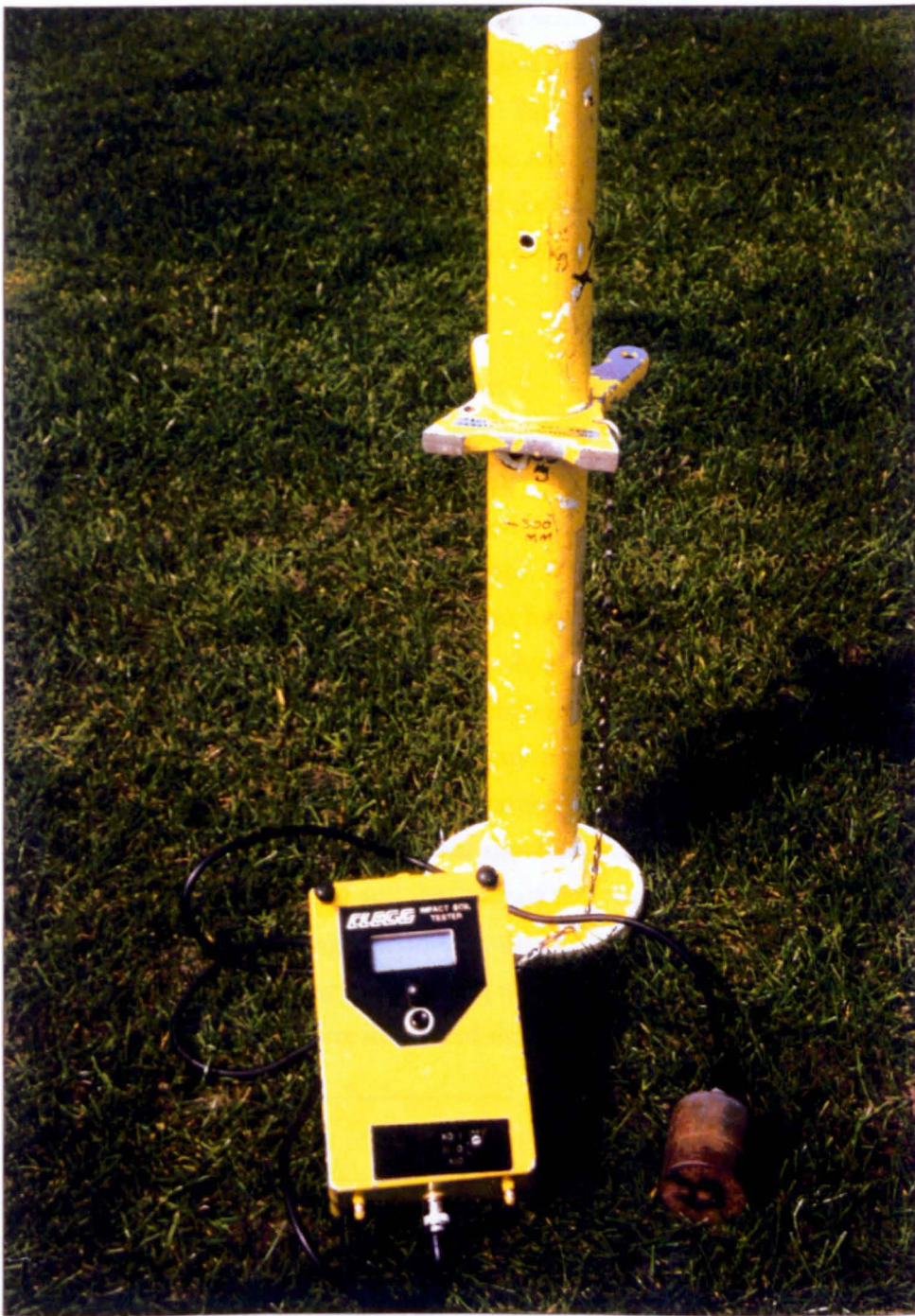
PLATE 4. Clegg Impact Soil Tester used for measurements of hardness. The plate shows the 0.5 kg test mass containing an accelerometer at the lower right, the meter unit at the lower left and the guide tube at the rear.
