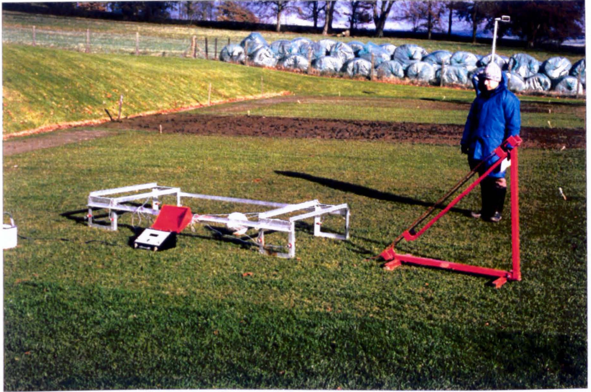
PLATE 3. The Author measuring ball deceleration on the experimental plots described in Section 3 of this chapter using the timing gate apparatus. The timing gates are at each end of the apparatus and the ball roll ramp is used to provide a standard initial velocity.
