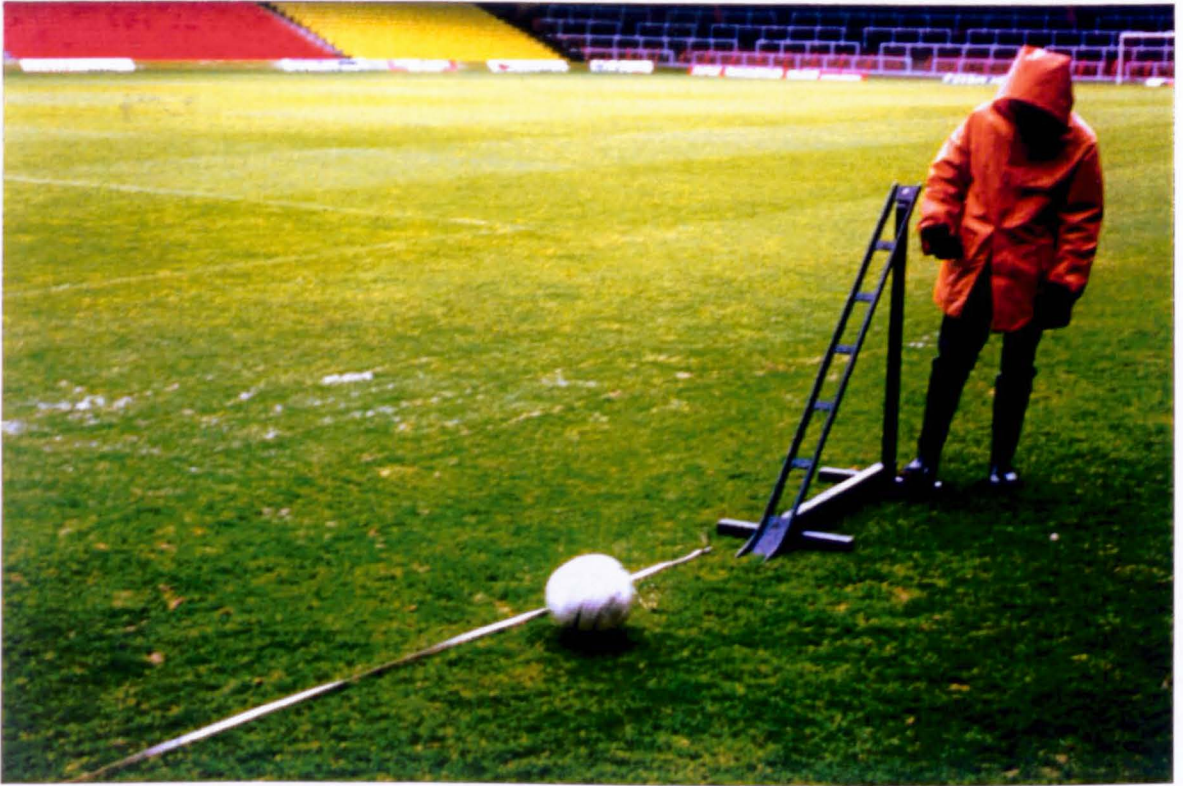
PLATE 2. Ball roll testing at Anfield Road, Liverpool.
