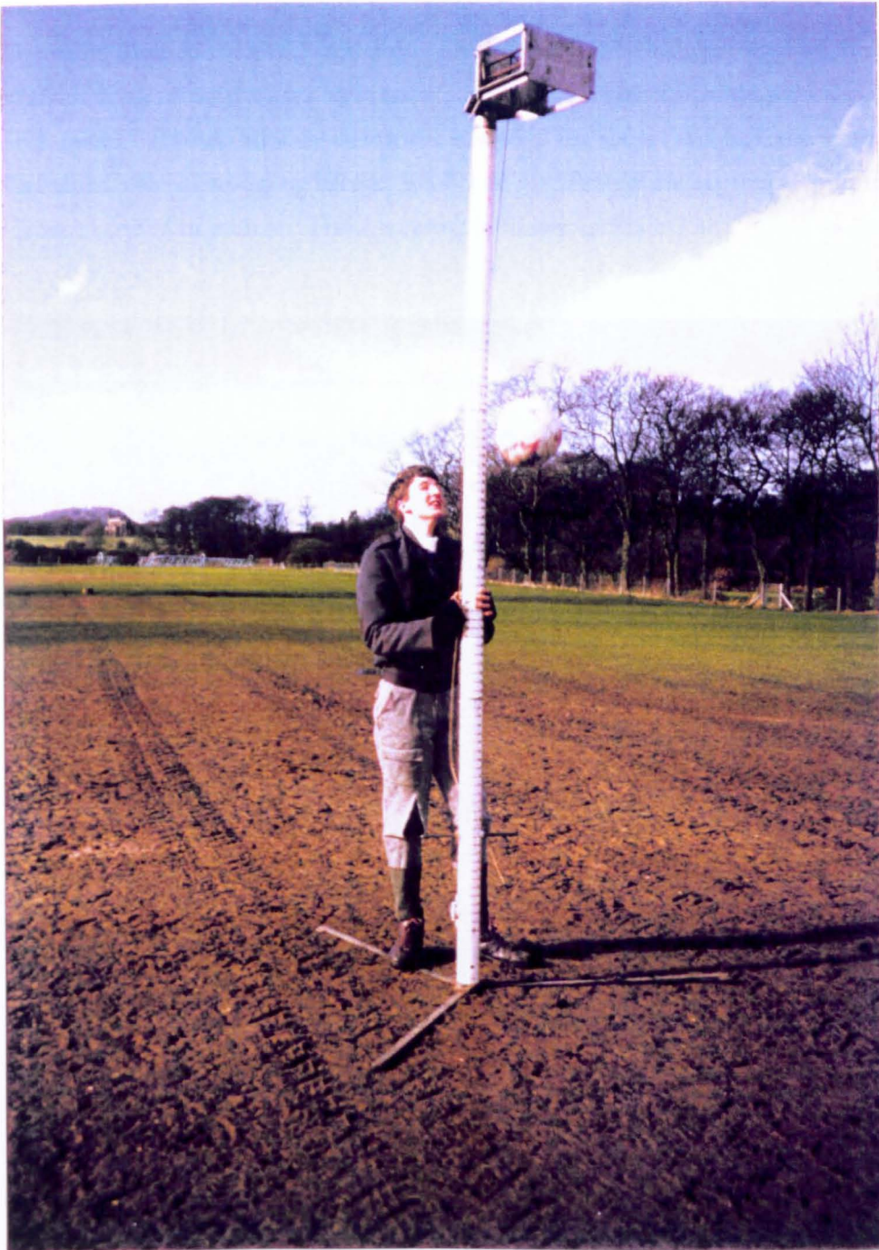
PLATE 1. Apparatus for measuring ball rebound resilience in use on a reinforced rootzone as described in Chapter 5.
