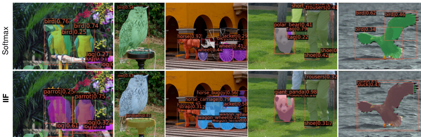
Fig. 4. MaskRCNN-ResNet50 detections on LVISv1 validation set using Softmax versus our IIF method. IIF can correctly detect rare classes such as parrot, owl, horse-carriage and giant panda in contrast to Softmax method. However, both methods fail to detect the rare class eagle in the last image.
