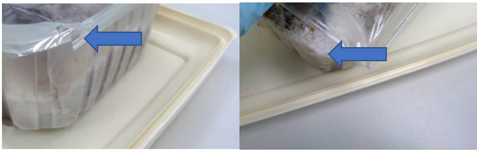
Figure 3.1: Shattered rigid plastic packaging and open film seal from samples from two different brands of RMD
