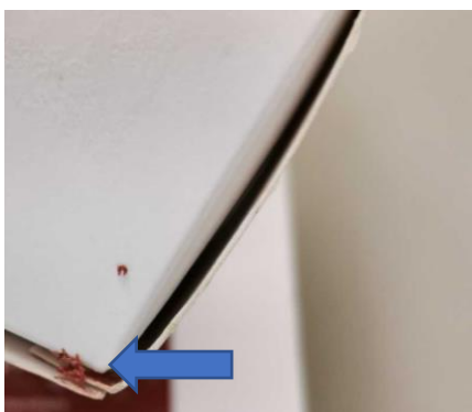
Figure 3.2: Frozen raw material evident on outside of cardboard packaging of RMD sample prior to defrosting
