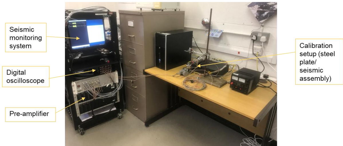
Figure 3.4: Calibration setup (steel plate or seismic assembly) connected to seismic acquisition apparatus for ball drop experiments.
