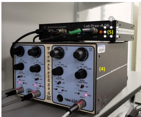
Figure 2.4. Uterine contractions. During contraction, the transducer recorded the variations in tension which was amplified through an amplifier (4) then converted into a digital signal by a converter device (5). C. Through an acquisition software, the computer recorded signals as expressed on the screen D (6)
