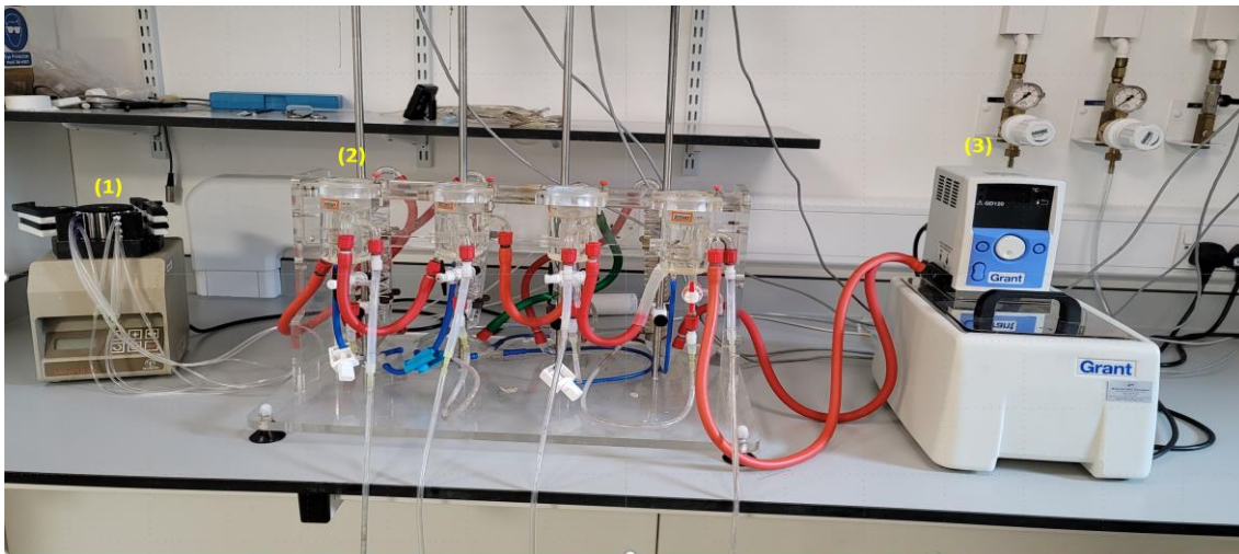
Figure 2.3 A. Organ bath. The myometrial strips were superfused in the organ bath with PSS by the way of a peristaltic pump (1). Strips were mounted vertically in an organ bath (2). The circulating water bath maintained the reservoir at a set temperature (3).
