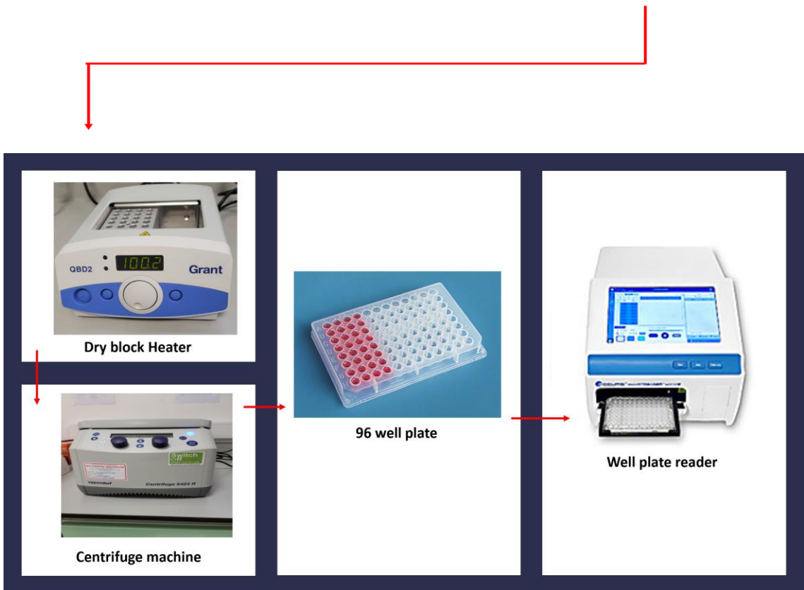
Figure 2.7 Glycogen measurement, tissue preparation procedure. Freeze-drying and homogenising processes, boiling and centrifugation. (Figure drawn by Tshikaya Kaleta)
