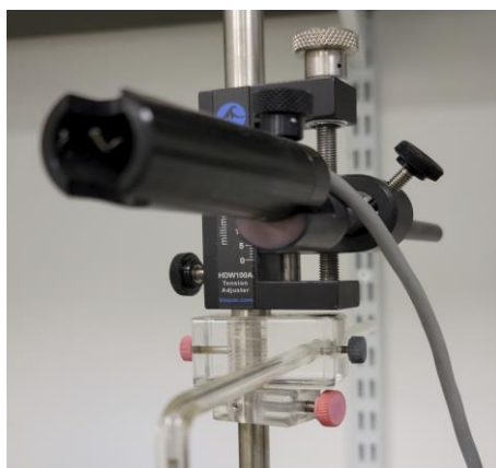
Figure 2.3. B. Force transducer. The contraction measurement was obtained by the mean of a force transducer (B).
