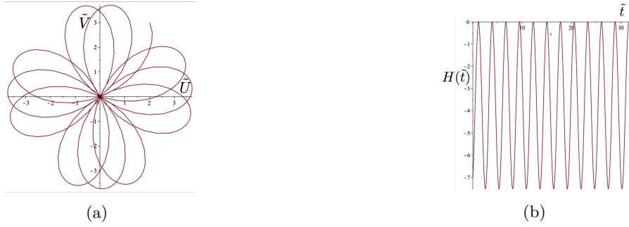
Figure 9: Class 2(b) example. (a) Trajectory of the gyropendulum with smooth loops passing through the origin and (b) the function H(\tilde{t}) with \Gamma = -1.077 and initial conditions \tilde{U}_0 = 2 , \tilde{V}_0 = 3 , \dot{\tilde{U}}_0 = 1 , \dot{\tilde{V}}_0 = -2 . The condition for Class 2(b) is satisfied with H(0) = \Gamma|\tilde{\mathbf{Q}}(0)|^2/2 = -7 . In addition H(\tilde{t}) \leq 0 .
