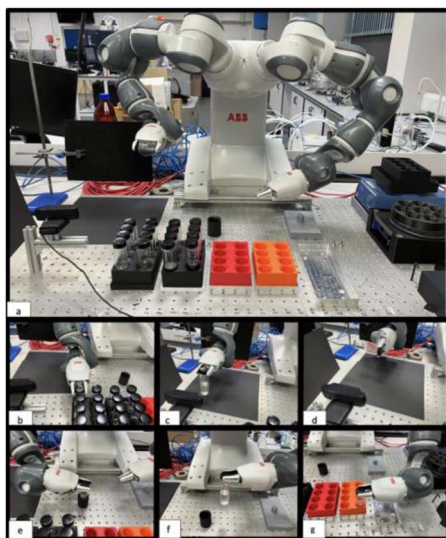
Fig. 1 Autonomous testing of viscosity using a dual-arm robotic platform. (a) Photograph showing the whole autonomous platform. (b) First, the right-hand arm picks a sample from one of two analysis racks; (c) next, the same arm moves the sample to a camera station; (d) the robot rotates the sample through 90° at a pre-defined velocity while capturing video data. (e) Following video acquisition, the right-hand arm places the vial into the transit holder. (f and g) The left-hand arm then moves the vial from this transit holder and places it into one of two storage racks.
