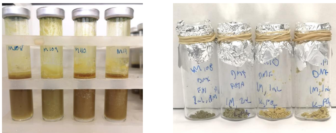
Figure 258: Al:STO/DBTS-DBTS Hybrid samples containing 10 wt.% Al:STO synthesised from various DMF:[ K_3PO_4 ] reaction solutions. a) Hybrids dispersed in reaction mixture after completion of the microwave-assisted polycondensation reaction, b) Hybrid samples after isolating, washing, and drying.
