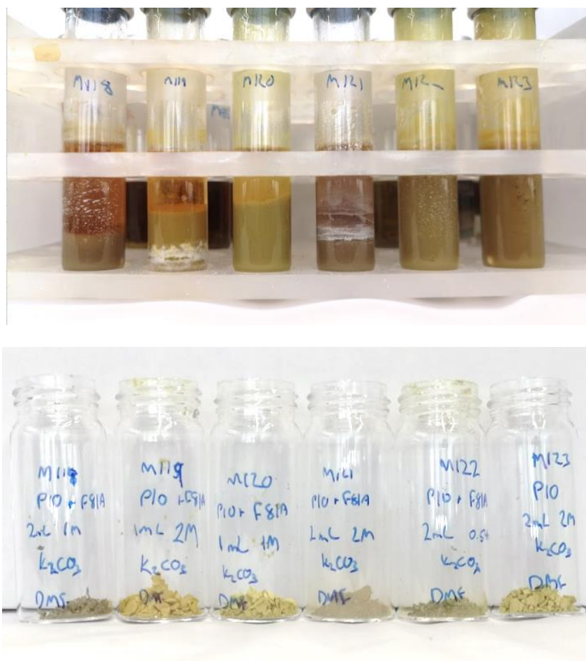
Figure 255: \text{RhCrO}_x@/\text{Al:STO}/\text{DBTS-DBTS} hybrids containing 10 wt.% Al:STO synthesised in \text{DMF}/\text{K}_2\text{CO}_3 reaction mixtures with various solvent/base volume ratios and base concentrations See Table 26 for details. a) Reaction mixtures following microwave synthesis, b) Samples after being isolated, washed with water and MeOH and dried in a vacuum oven overnight.
