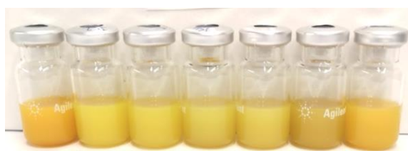
Figure 176: Top) HER rates and synthesis yields for BDT-PhFx polymers synthesised from a toluene/K 2 CO 3 reaction mixture. Bottom) Image of 5 mg of same BDT-PhFx polymers dispersed in 5 ml of 1:1:1 TEA/MeOH/H 2 O solution.
