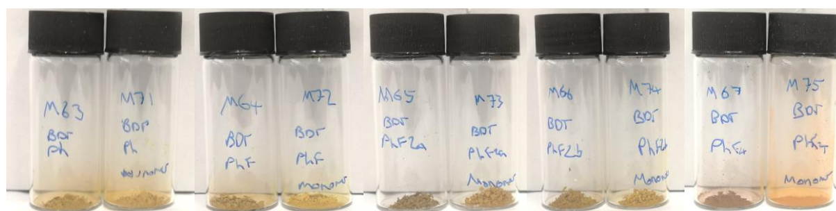
Figure 182: Photographs of products resulting from attempted synthesis BDT-PhFx-Br 2 monomers and the DBT-PhFx polymers synthesised from stoichiometric mixtures of BDT-PhFx. Reactions were performed under similar conditions with the exception that monomers were synthesised at 100°C whereas polymers were synthesised at 120°C.
