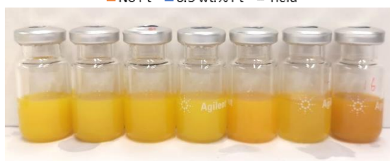
Figure 175: Top) HER rates and synthesis yields for BDT-PhFx polymers synthesised from a dioxane/TBAA reaction mixture. Bottom) Image of 5 mg of BDT-PhFx polymers dispersed in 5 ml of 1:1:1 TEA/MeOH/H 2 O solution.
